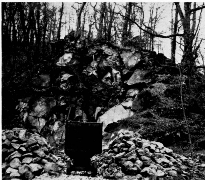
FIGURE B.—Small olivine quarry in large residual boulders of dunite.
