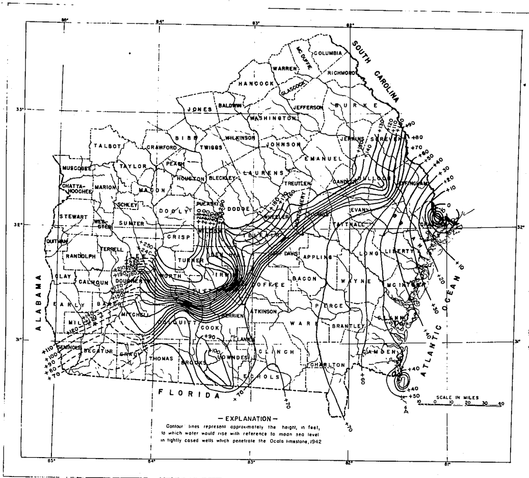
Figure 2. Map showing piezometric surface of artesian water in the principal limestone aquifer in southern Georgia.
