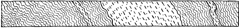
Cross-section through the Worley Gold Mine, Cherokee County, Georgia, Showing Auriferous Quartz Veins in the Crystalline Schists, Indicated by dots and Broken Lines.
