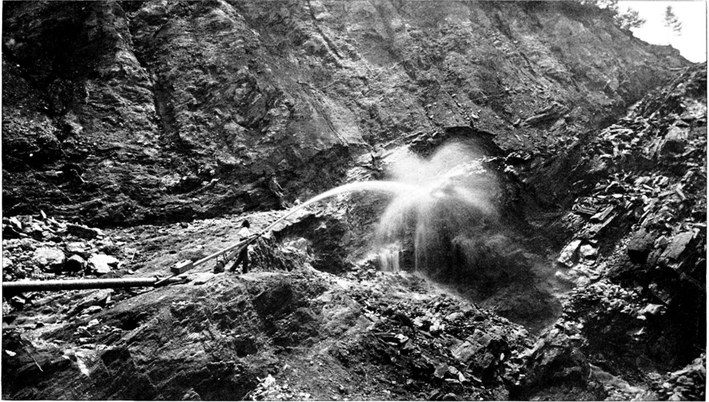
HYDRAULIC MINING IN THE DECOMPOSED AURIFEROUS SLATES, WITH THEIR VEIN CONTENT, AT THE SINGLETON MINE, DAHLONEGA, GEORGIA.
