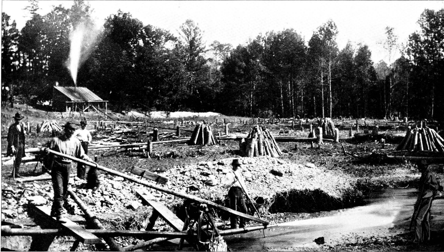
HYDRAULIC GIANT IN OPERATION, ON THE PLACER PROPERTY OF THE MICHIGAN GOLD MINING CO., NEAR BURNT HICKORY PAULDING COUNTY GEORGIA.
