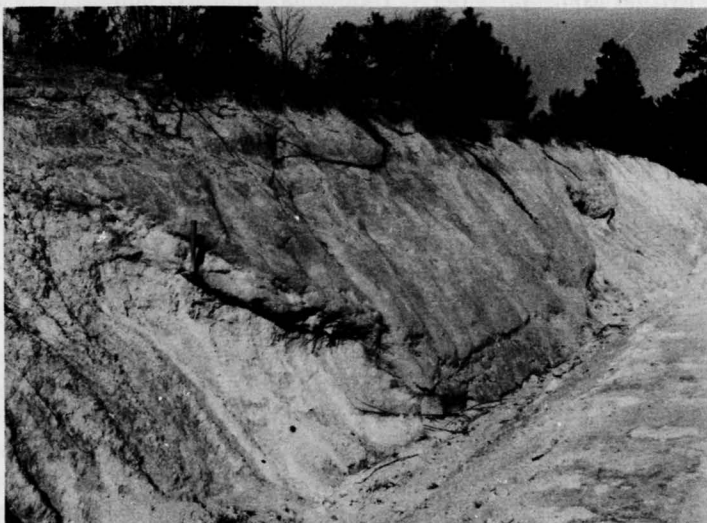
FIGURE 4. Exposure in road cut 1 mile east of Black Springs Church on Georgia Route 22 (Baldwin County) showing pink coarse sand filling a channel in deeply weathered granite.
