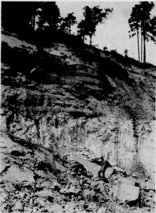
FIGURE 6. Stevens Pottery kaolin mine, 5.7 miles north of Gordon on Stevens Pottery-Gordon road (Wilkinson County). White kaolin of the Tuscaloosa formation overlain unconformably by 40 feet of calcareous sand and clay of the Barnwell formation.
