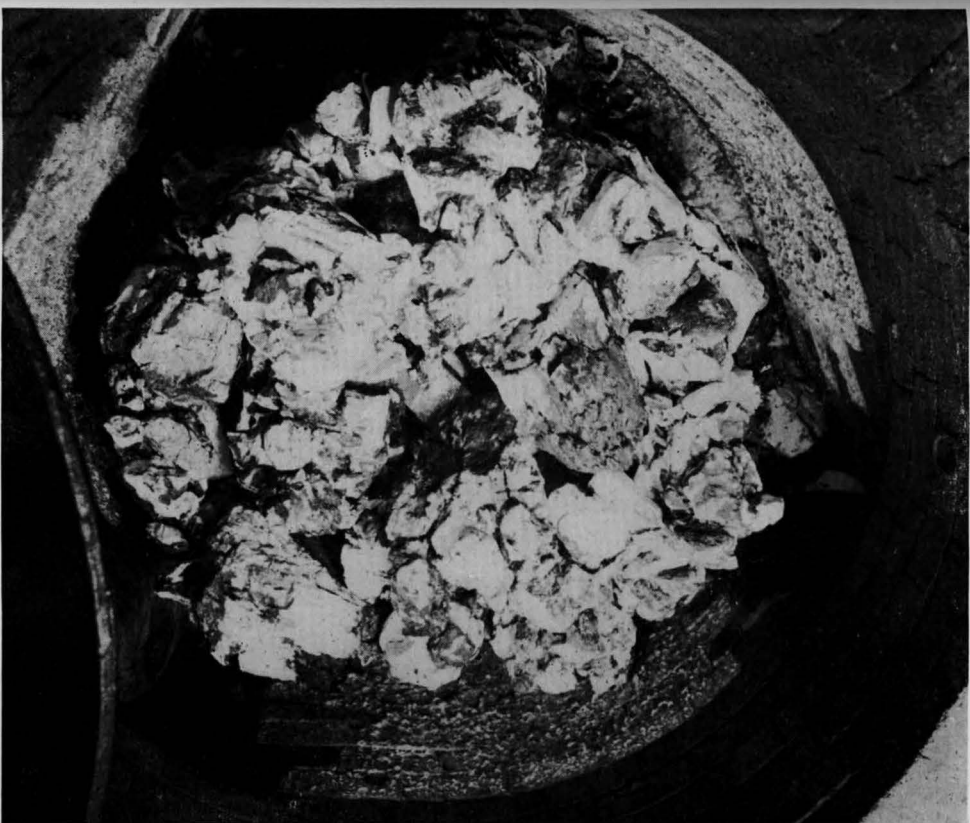
Figure 15. Top view of pile of Georgia massive kyanite lumps after heating to 1600^{\circ} C. in a round oil-fired kiln. Three slagged areas on side walls show position of silicon carbide brick.
