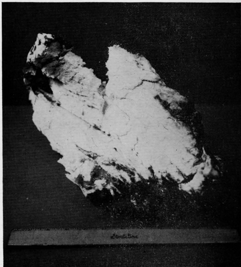
Figure 19. One-half of this lump split and fell off during firing leaving the white interior exposed. The top left portion has fallen away in a pyroplastic fashion from a position of alignment with the central pinnacle.
