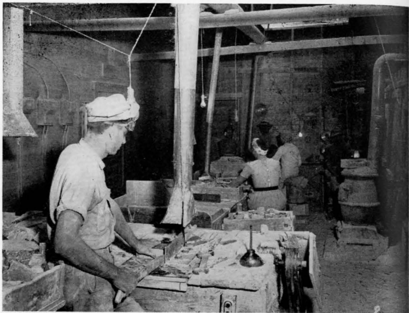
Figure 9. Crayon saw line; stock saw in foreground, with crayon saws in background. Note dust collectors above each saw. Facing and cut-off saws not shown.
