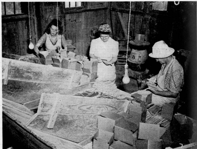
Figure 10. Grading and packing talc crayons. A gross is packed in each box.
