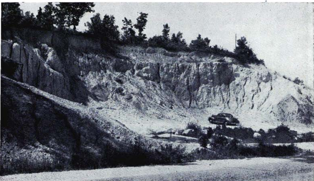
Fig. 14. Chert quarry (road surfacing material) U. S. Hy. 27, two miles south of Summerville, Chattooga County, Georgia.
