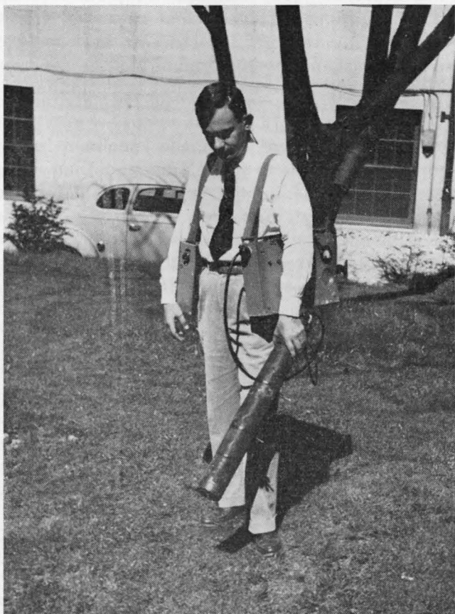
Figure 7. The Field set in use. The small unit under the right arm contains a high voltage supply for the Geiger-Mueller tube.
