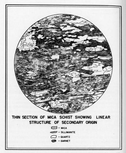
Figure 4. Sketch of a thin section of foliated schist. The cleavage direction is from left to right parallel with the sillimanite needles. Micas are shaded with different intensity in agreement with the colors of the grains in the section.
