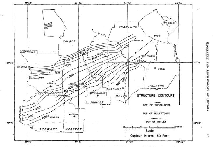
Figure 6. Structure contours on tops of Tuscaloosa, Blufftown, and Ripley formations.
