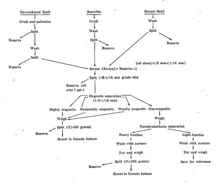
Figure 1—Flow sheet for sample treatment.
