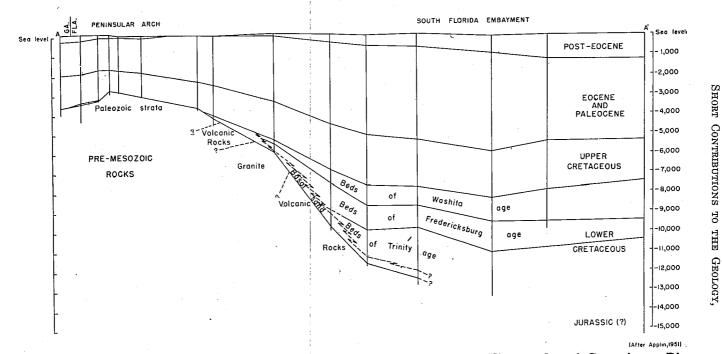
Figure 3. Geologic cross section extending south from the crystalline rocks of Georgia to Big Pine Key, Monroe County, Florida.
