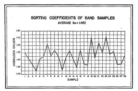
Figure 3. Range of sorting coefficients for the twentyeight samples. The average is representative of a well-sorted deposit.
