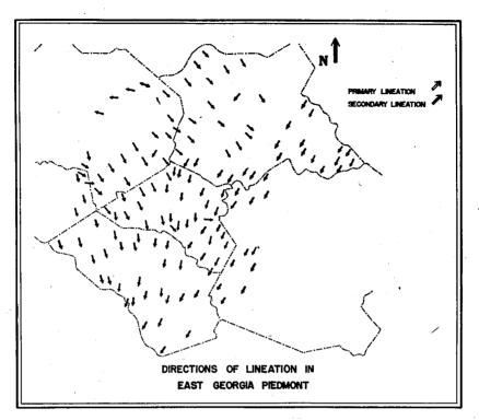
Figure 2. Linear directions in mapped area of east Georgia Piedmont. Note the similarity in trends between primary and secondary lineations.
