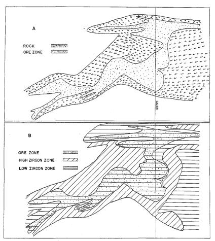
Figure 4 Calloway Mine 14 Level A. Ore Outline as Projected Before Heavy Mineral Study. B. Ore Outline as Projected After Heavy Mineral Study.
