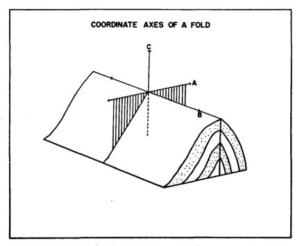
Figure 3. Sketch of a fold showing the assumed positions of the a, b, and c coordinates (after E. Cloos).
