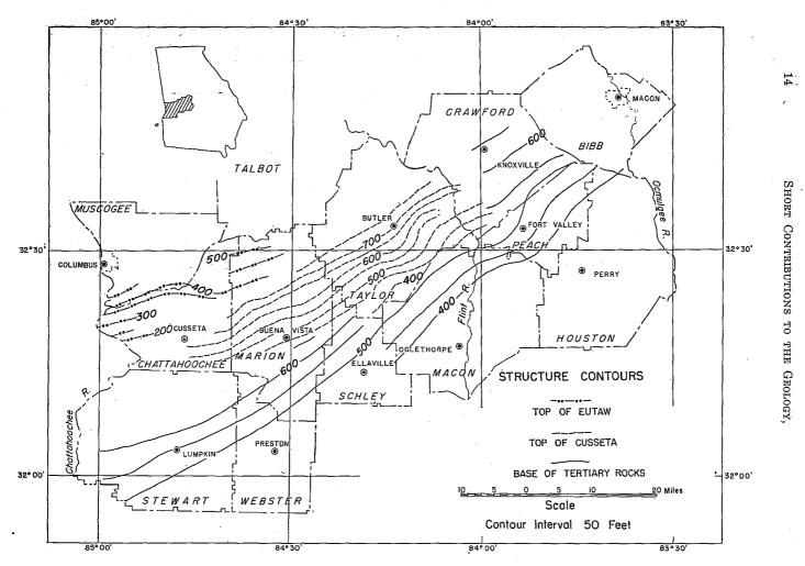
Figure 7. Structure contours on tops of the Eutaw formation and the Cusseta sand, and on base
