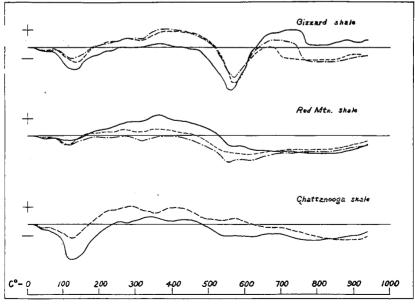
Figure 3. Thermal Analysis of Shales.
