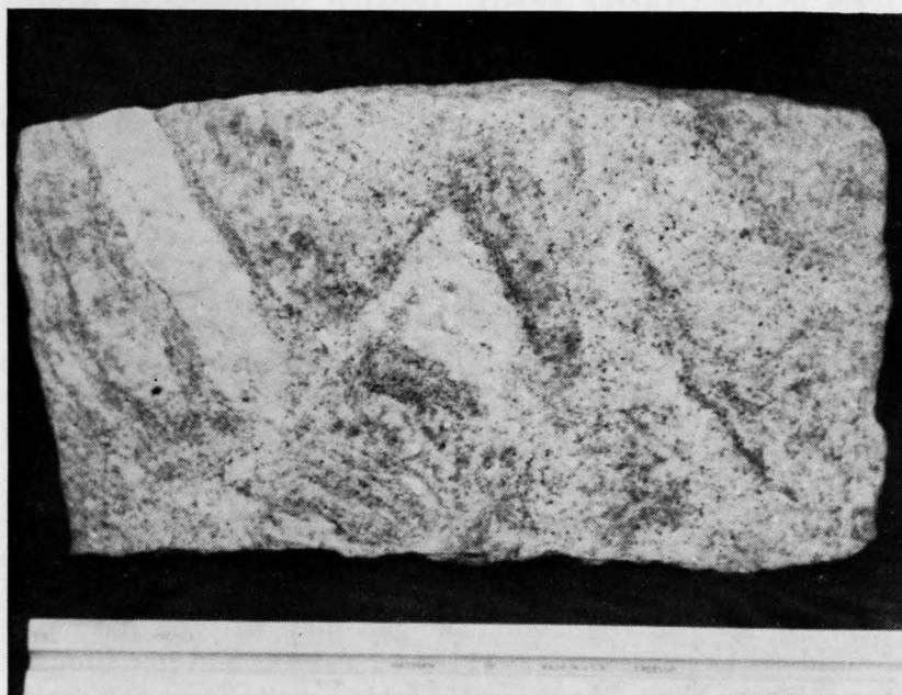
Fig. 17. Shear zone in building block of the Lithonia gneiss. Displacement of banding and aplite vein approximately four inches.
