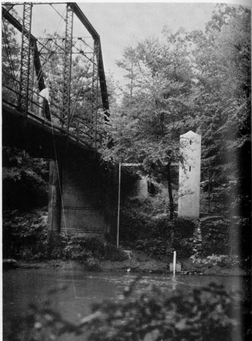
Figure 10. Typical stream gaging station. Water measurement being made at station on South River near McDonough, Georgia.
