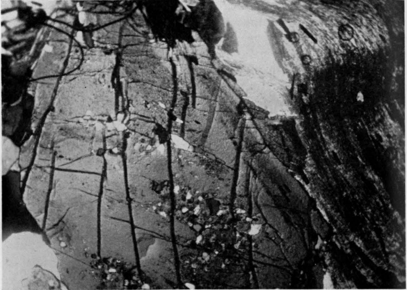
Figure 5.—Staurolite crystal and folded mica in staurolite-mica schist. Crossed nicols 35 X. Rock from road cut 0.6 miles northwest of Bethany Church.
