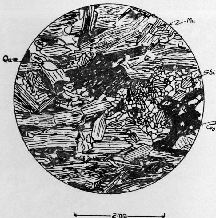
Figure 9.—Muscovite schist containing muscovite (Mu), quartz (Qu), iron oxides (FO) and sillimanite (Si) relics. Rock from road cut 150 feet north of the intersection of Georgia highway 171 and Cedar Creek.
