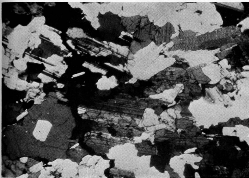
Figure 13.—Fractured plagioclase in muscovite granodiorite. Crossed nicols. 35X Rock from 2 miles S72W of Eagle Grove School.
