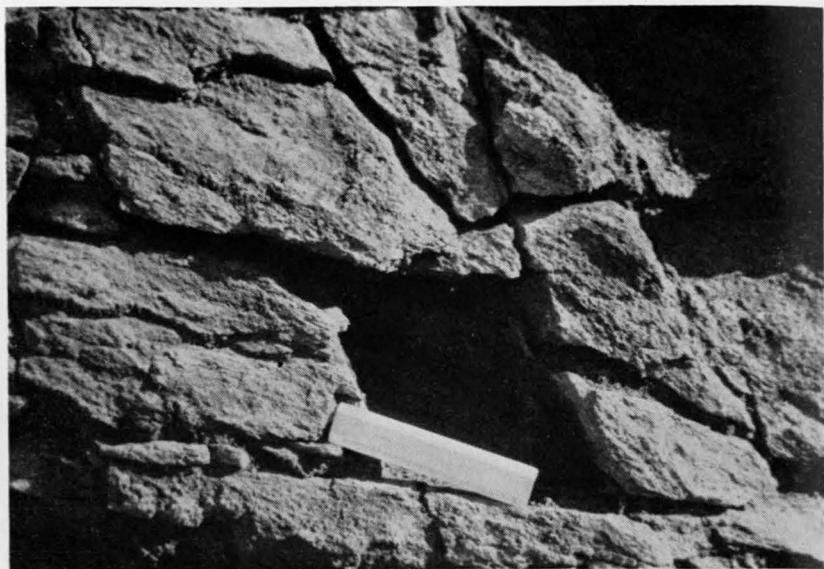
Figure 24.—Details of joint surfaces. The cleavage ( S_3 ) departs from the foliation ( S_2 ), (parallel to the ruler) at a slight angle.
