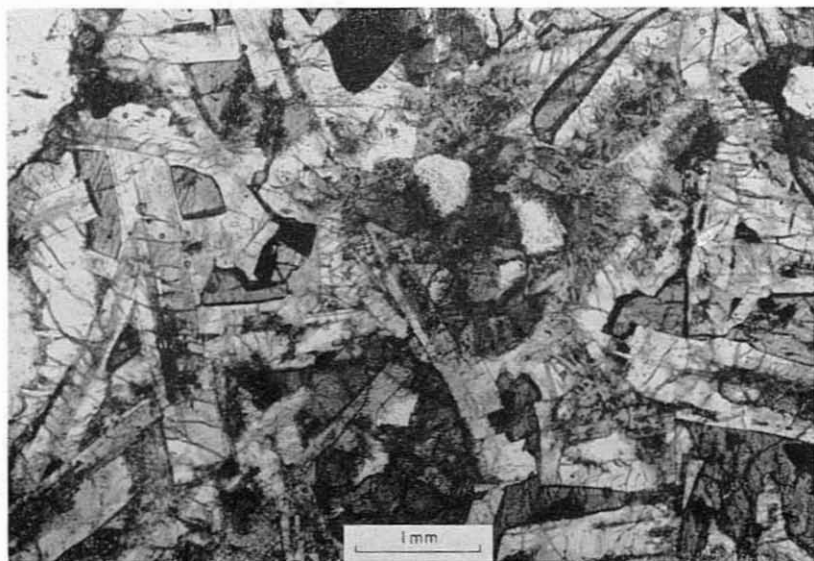
Figure 22. Thin section, plane-polarized light; Pulaski County, Georgia, Ainsworth Tripp No. 1, 2,675-2,684 ft.
