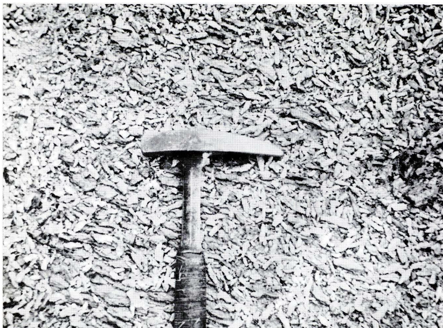
Fig. 12. Sheared Palmetto Granite, spindles released on weathering, about 2 miles south of the Fulton County Airport.
