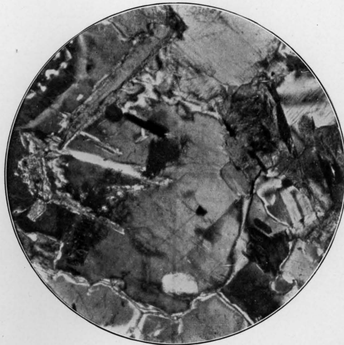
PHOTO-MICROGRAPH OF STONE MOUNTAIN GRANITE, FROM STONE MOUNTAIN, DEKALB COUNTY, GEORGIA. BETWEEN CROSSED NICOLS X 75.
