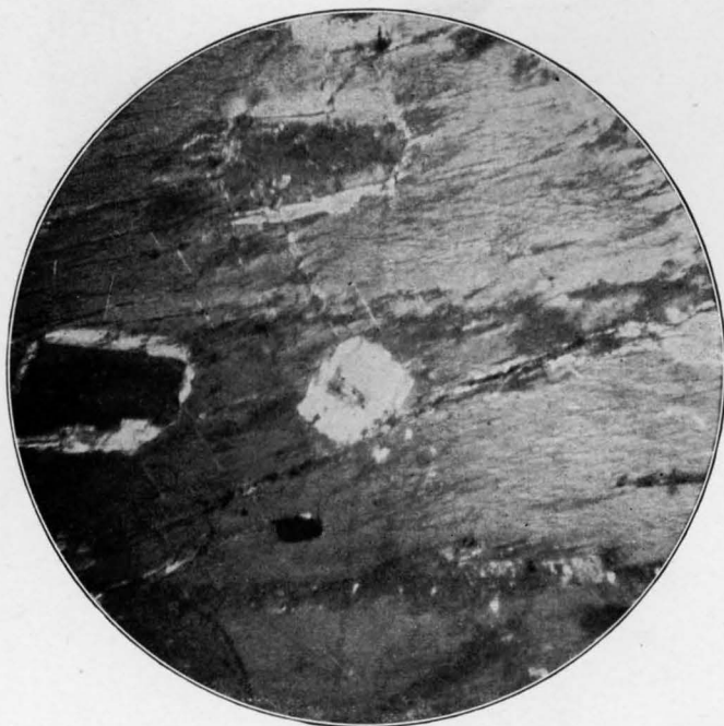
FIG. 2. PHOTO-MICROGRAPH OF A PHENOCRYST OF MICROPERTHITIC ORTHOCLASE, SHOWING INCLUSIONS OF QUARTZ, PLAGIOCLASE, BIOTITE, AND VERY SMALL PRISMS OF APATITE, FROM THE GRANITE OF FIG. 1.
