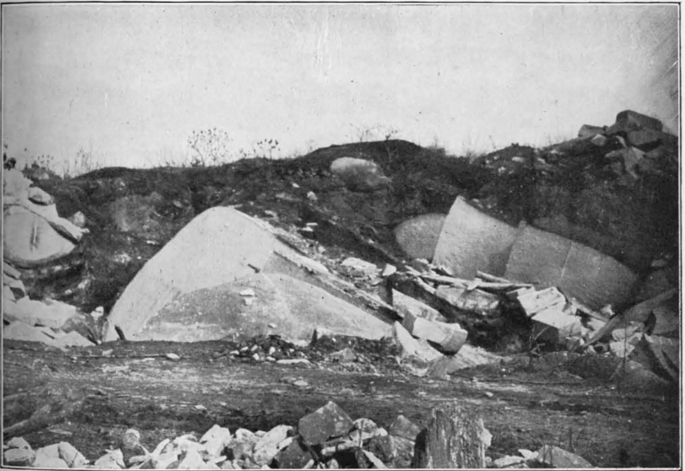
VIEWS IN THE COGGINS GRANITE QUARRY, OGLESBY, ELBERT COUNTY, GEORGIA. Fig. 1 Shows the Decayed Dark-blue Granite Overlying the Fresh Rock. Fig. 2 Illustrates the Spheroidal Weathering of the Granite.
