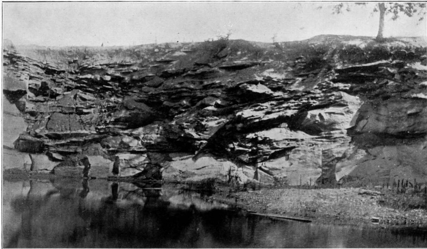
THE COLE QUARRY NEAR NEWNAN, GEORGIA, SHOWING, IN VERTICAL SECTION, GRANITE WEATHERING FROM THE LOOSE SOIL AT THE TOP, THROUGH THE PARTIALLY DECAYED, TO THE FRESH GRANITE, THE DECAY HAVING PROGRESSED ALONG HORIZONTAL LINES.
