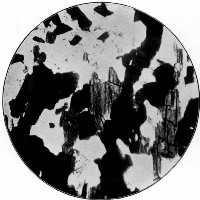
FIG. 1. PHOTO-MICROGRAPH OF HORNBLLENDE-GNEISS (AMPHIBOLITE), FROM THE T. B. TIGNER QUARRY, ON THE MACON & BIRMINGHAM R. R., MERIWETHER COUNTY, GEORGIA, x 74.
