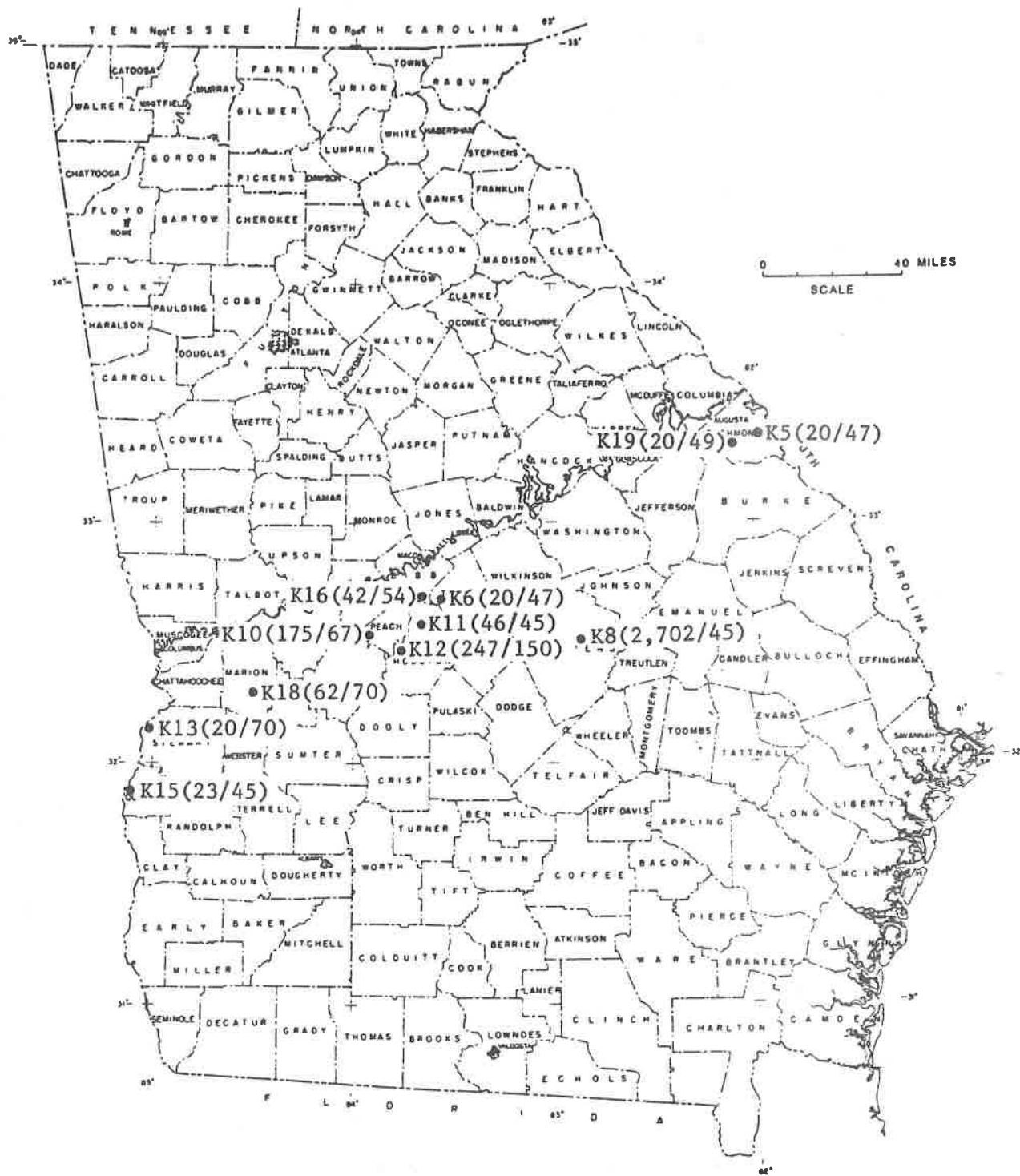
Figure 3-3: Water Quality of the Cretaceous Aquifer System: Metallic Cations Iron + Manganese (ppb)* / Copper + Lead + Zinc (ppb) (The minimum detection limit of Iron + Manganese = 20ppb. The minimum detection limit of Copper + Lead + Zinc = 45ppb.)
