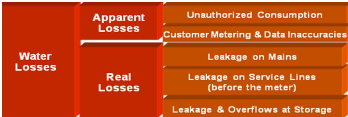
Figure 1: IWA/AWWA Water Audit Method and Apparent vs. Real Losses
