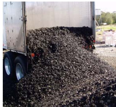
Tire chips are used to make other products, such as road base, or are burned in power plants as a source of fuel.
