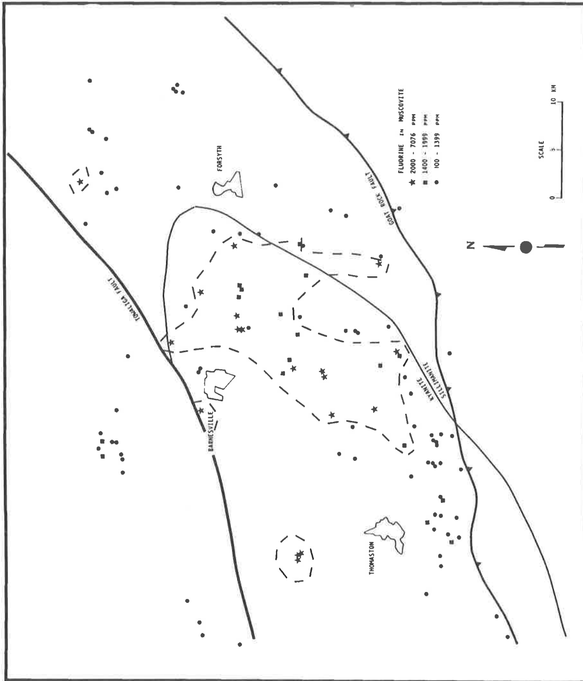
Figure 22. Map of the distribution of F in muscovite. Results (Appendix II) indicate that the highest F values (stars and squares outlined by the dashed line) occur mainly in the central part of the district and in the Indian Grave field to the northwest. The location of the kyanite-sillimanite isograd, the Towaliga and Goat Rock faults are shown for comparison.
