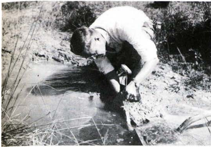
Fig. 13. A portable weir used to measure the flow of a very small stream. The weir has a sharp-edged notch through which the water flows. By measuring the depth of water in the notch, as shown, an accurate measurement of small flows can be obtained.
