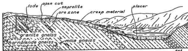
Figure 2.—Diagrammatic cross-section of a North Georgia stream valley showing the relations of lode, saprolite, and placer. (After G. W. Crickmay.)
