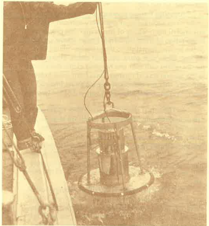
FIGURE 2 - Static underwater gamma detection system. Base of unit must be in direct contact with seafloor to register readings for spectrum analysis.
