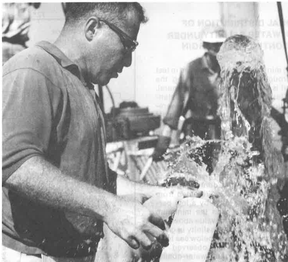
Figure 1. The natural freshwater flow from JOIDES test hole J-1B, 40 km offshore from Jacksonville, Fla., being sampled by G.W. Leve, U.S. Geological Survey. The top of the pipe protrudes through the drilling hole in the center of the Caldrill drilling vessel to about 5 m above sea level. The bottom of the drill pipe was set opposite Eocene limestone about 250 m below sea level at the time of the photograph. Photo by R.L. Wait, U.S. Geological Survey.
