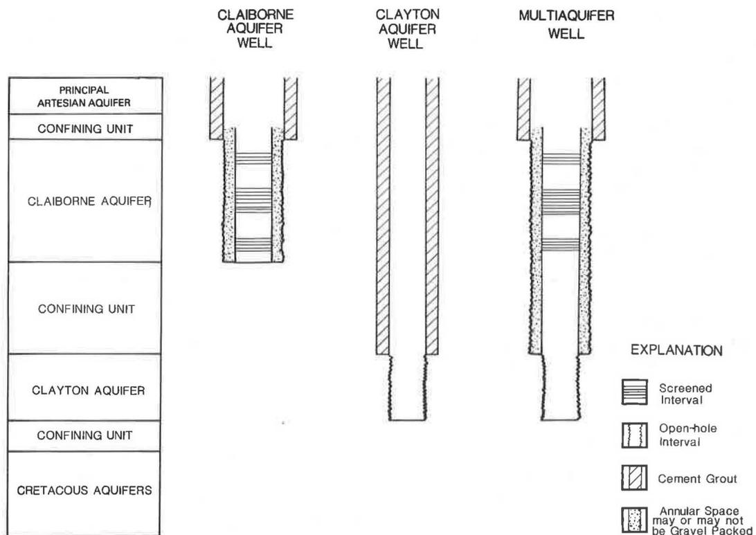
Figure 13. Typical Well construction in the Study Area.
