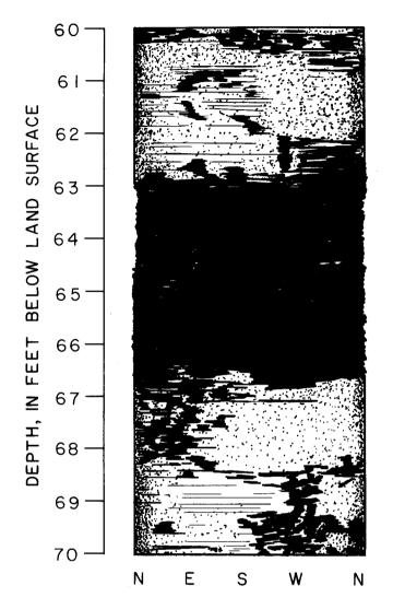
Figure 5. Televiewer image of waterbearing fracture and weathered zone eroded by drill, test well 3 (9DD1). Letters at bottom of image refer to compass quadrants.
