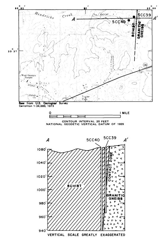
Figure 25. Well in contact zone between schist and granitic gneiss. Well 5CC39 yields 100 gallons per minute from the contact zone. Well 5CC40, which missed the contact zone, supplied about 1 gallon per minute.
