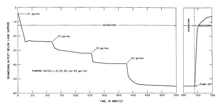
Figure 33. Drawdown and recovery curve for step drawdown test on test well 3 (9DD1).
