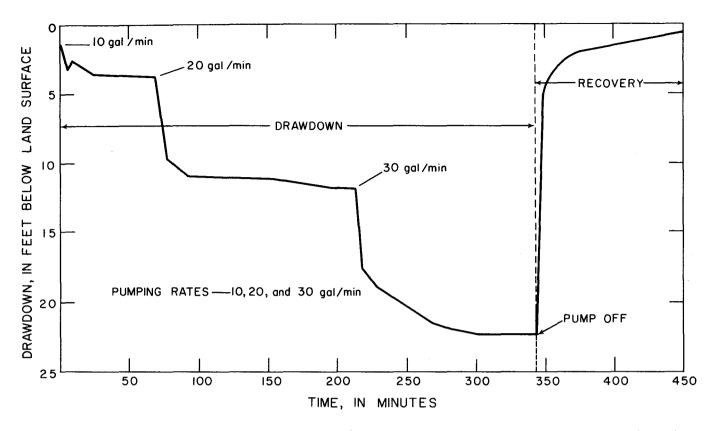
Figure 29. Drawdown and recovery curve for step drawdown test, test well 2 (8CC8).
