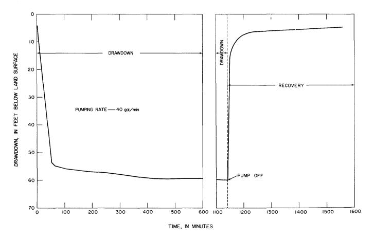
Figure 34. Drawdown and recovery curve for long-term pumping test on test well 3 (9DD1).
