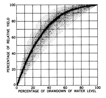
Figure 31. The curve shows that an increase in yield of a well is not directly proportionate to an increase in drawdown of the water level. A yield of nearly 80 percent of the total capacity of a well results from lowering the water level only 40 percent of the available drawdown. (LeGrand, 1967).
