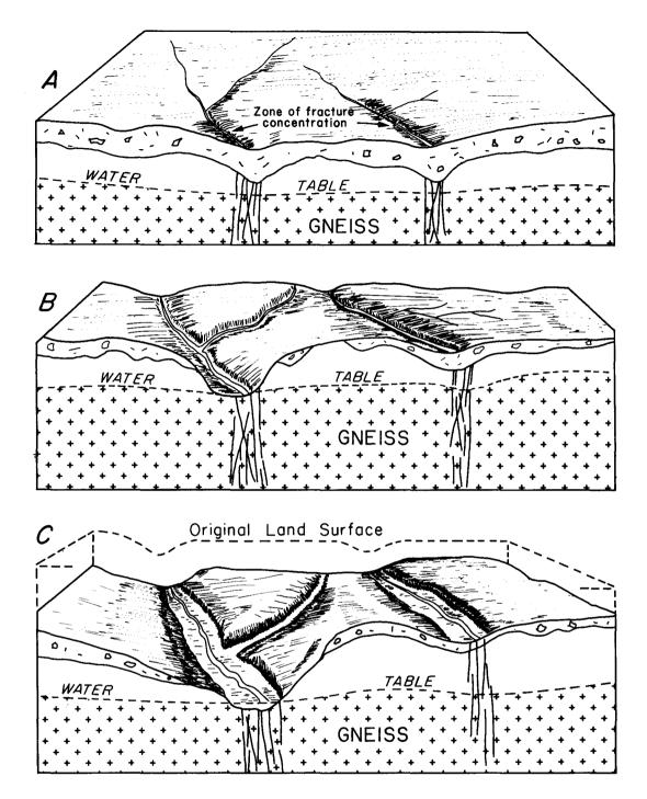
Figure 16. Valley development localized along zones of fracture concentration. Modified from Parizek (1971).
