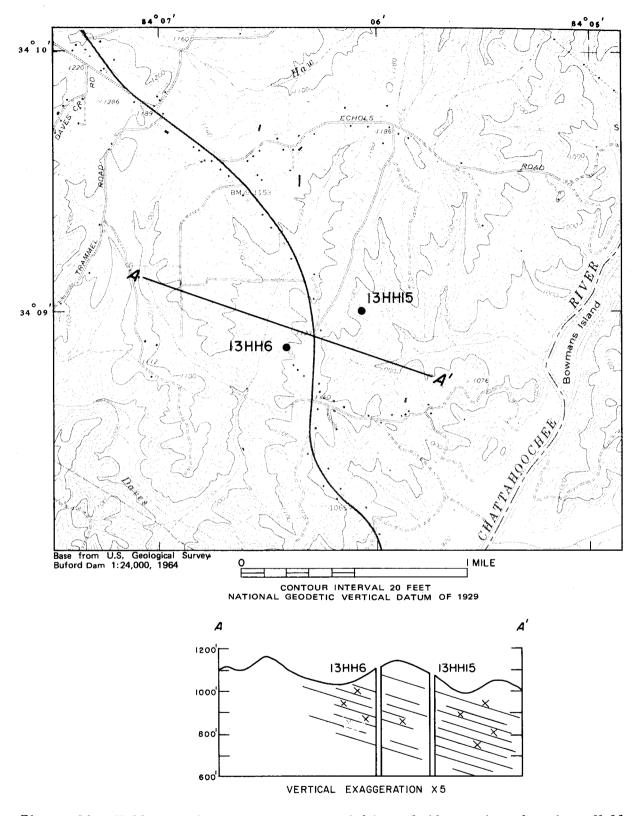
Figure 26. Wells tapping contact zones within multilayered rock unit. Well 13HH6 on downdip side of stream is 401 feet deep and yields 24 gallons per minute. Well 13HH15 is 660 feet deep and yields 6 gallons per minute.
