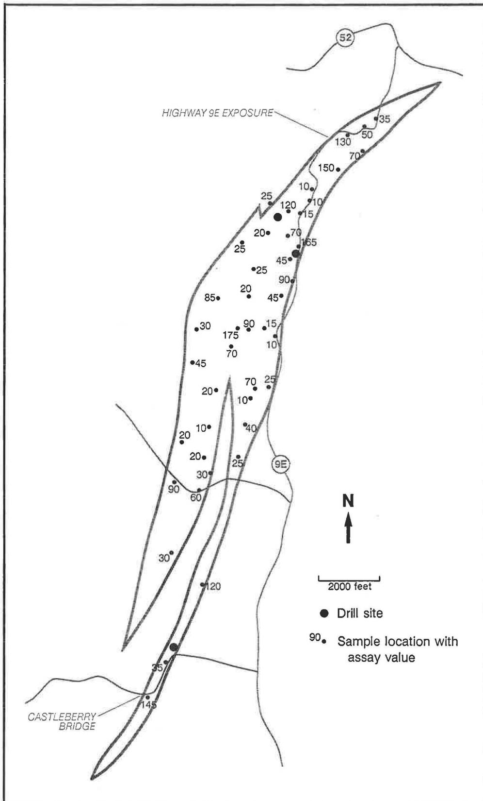
Figure 14. Reconnaissance geochemical survey for copper. Values are in ppm.
