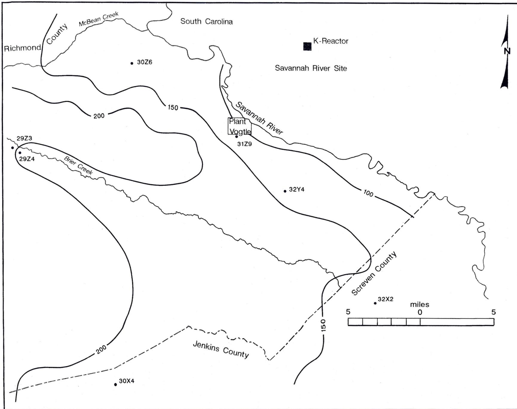
Figure 38. Potentiometric surface map of the Gordon aquifer, as defined by data from a larger regional study (modified from Brooks and others, 1985). Elevations are in feet above mean sea level. Wells are identified in Appendix 8.
