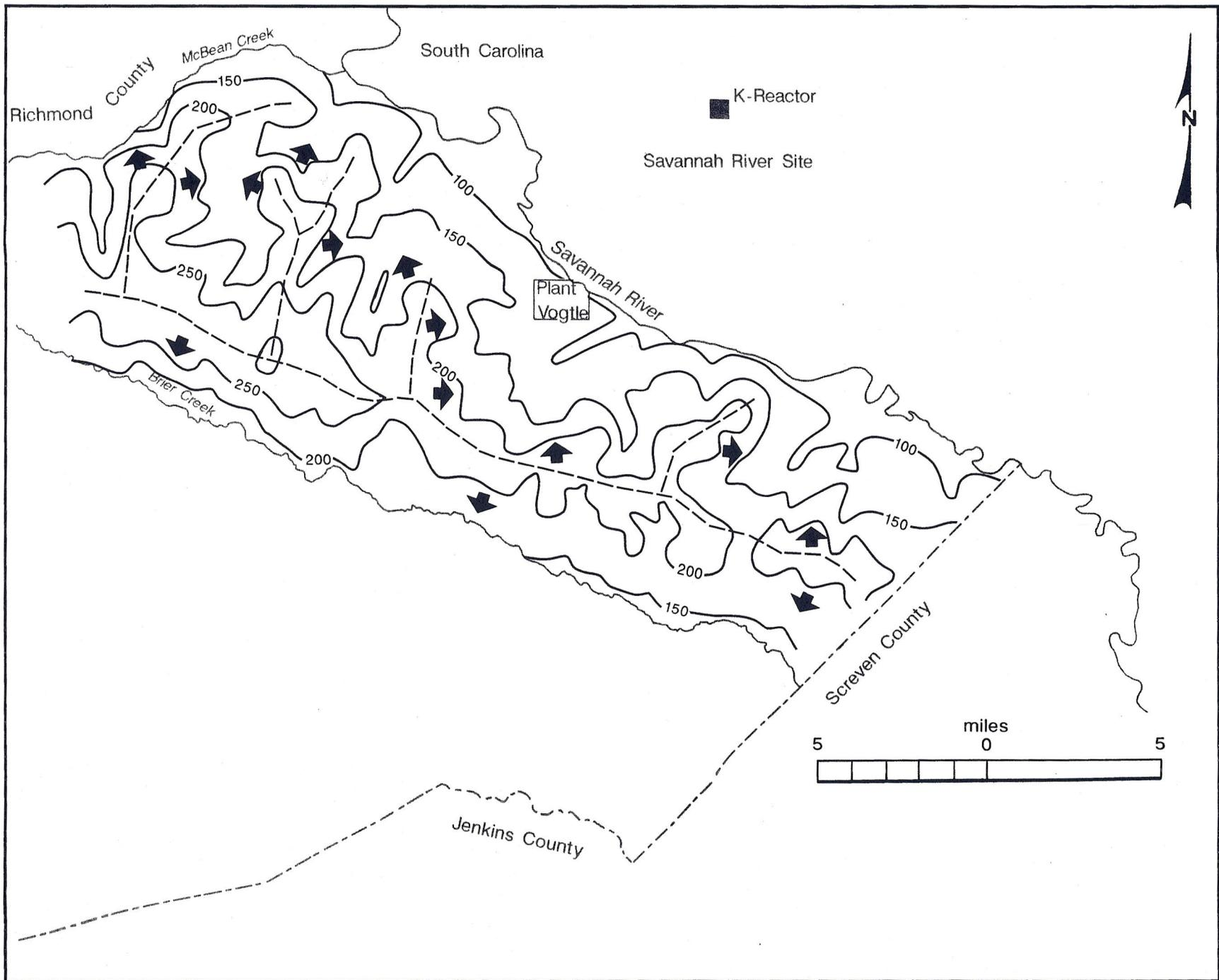
Figure 35. Water table surface map of the Upper Three Runs aquifer in eastern Burke County. Contours are in feet above mean sea level. Dashed lines represent ground-water "divides".
