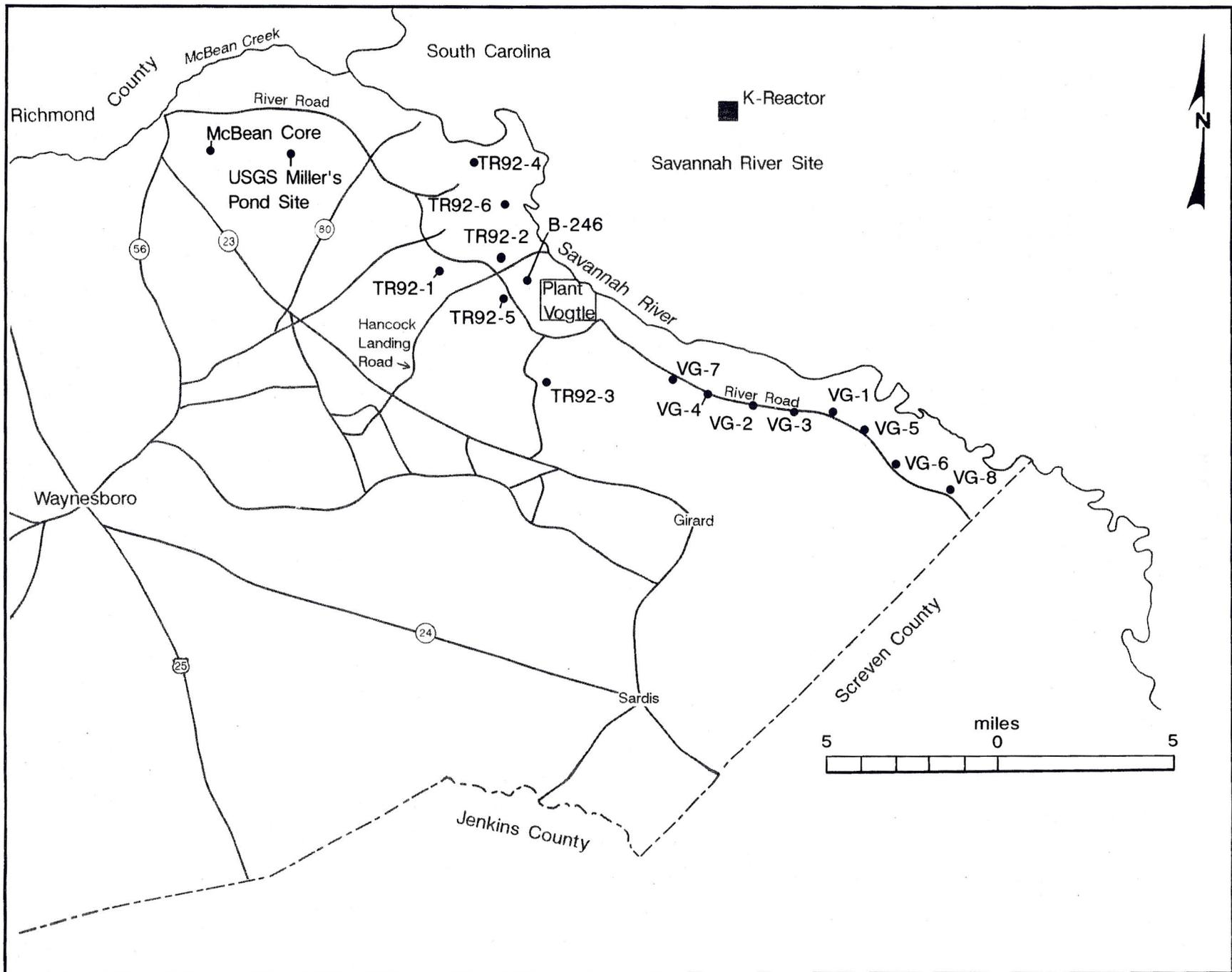
Figure 21. Index map of eastern Burke County, showing locations of cores used to develop the geologic framework. Core B-246 was drilled by Georgia Power in the early 1970's. "VG" cores were drilled by the Bechtel Corporation in 1982. All other cores were drilled by GGS.
