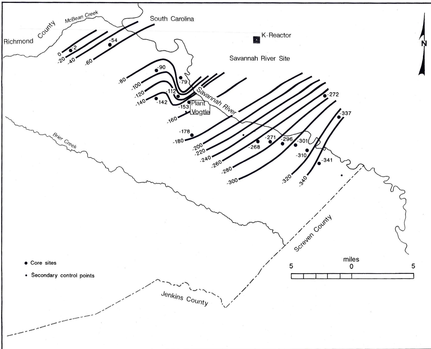
Figure 34. Structural contour map on the top of the Steel Creek Formation. Elevations are in feet relative to mean sea level.
