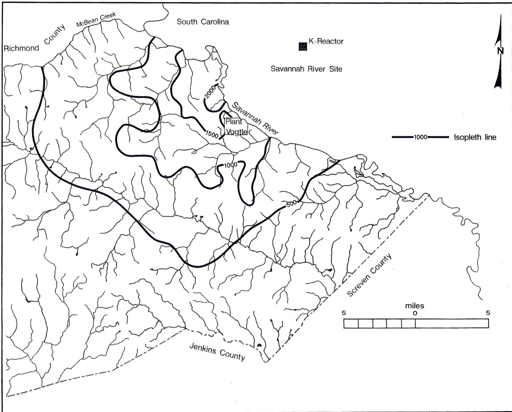
Figure 26. Isopleth map based on surface water tritium values of the 1992 base flow study, eastern Burke County. Values are in pCi/L.
