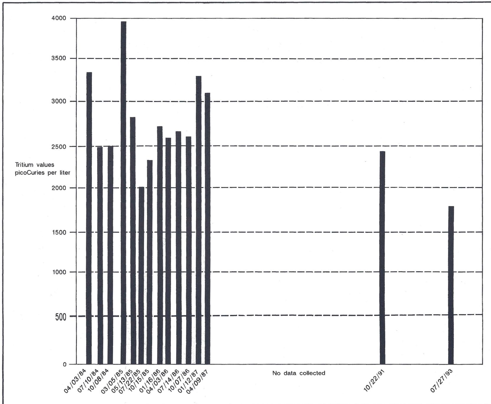
Figure 12. Bar graph showing tritium values in samples collected from Plant Vogtle spring at river mile 150.9. Values are shown in Table 4. Location is shown in Figure 11.
