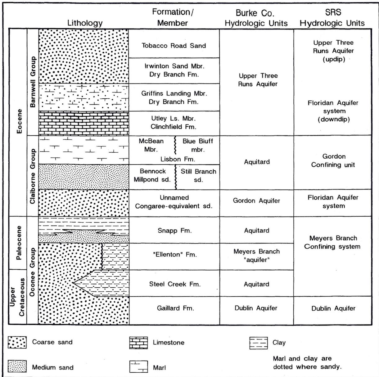
Figure 2. Stratigraphic and hydrostratigraphic units for Burke County and SRS area. SRS terminology from Aadland and others, 1992.
