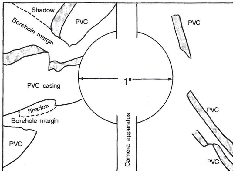
Figure 24. Photograph of the shattered portion of the Delaigle Trailer Park Well #3.
