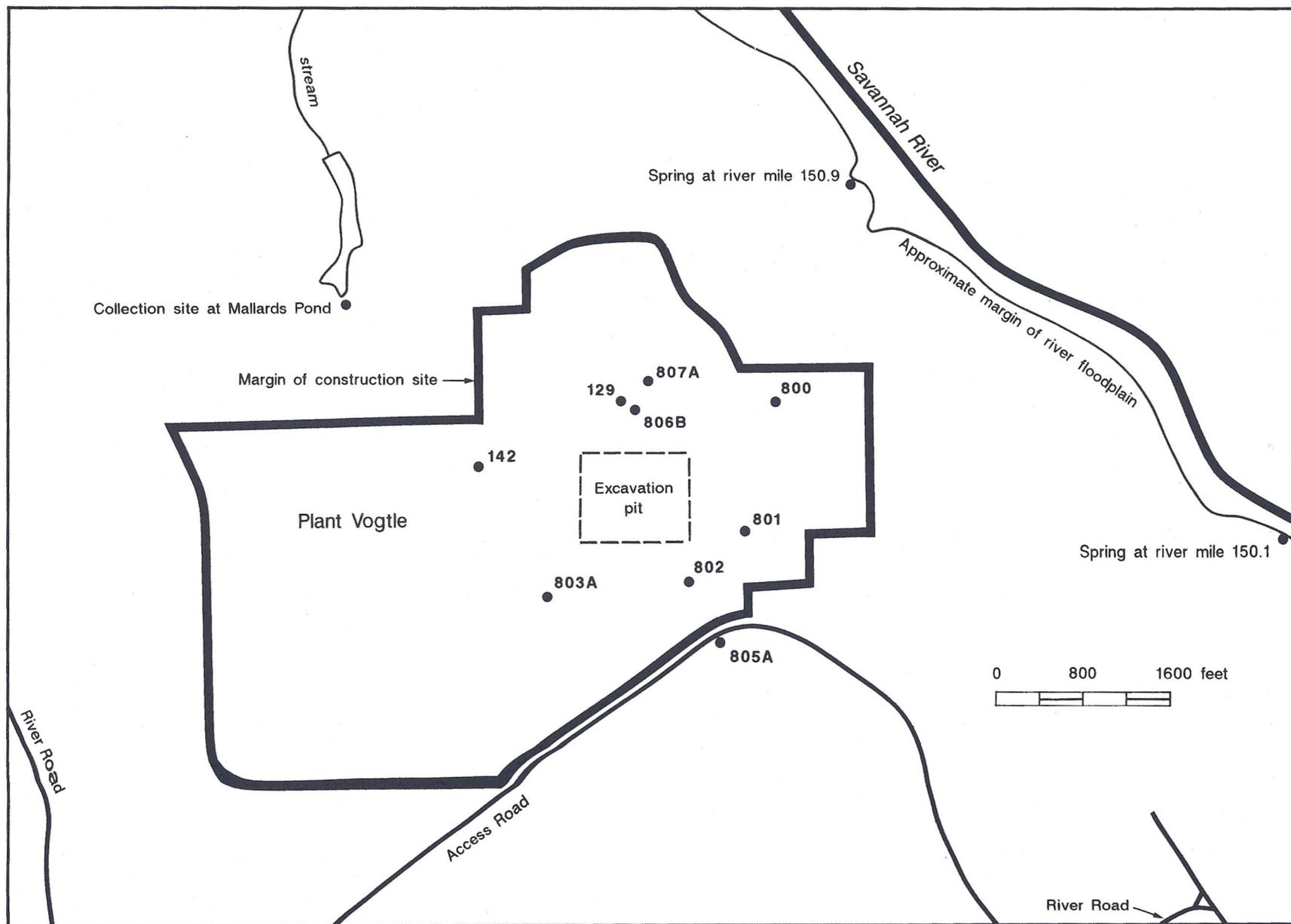
Figure 11. Map of Plant Vogtle construction site showing surface water collection sites and Upper Three Runs aquifer monitoring wells (1985 - 1991): refer to Tables 4, 5, and 6. (Modified from Georgia Power Co. Figure 2.4.12-2 - Plant Vogtle Final Safety Analysis Report.)
