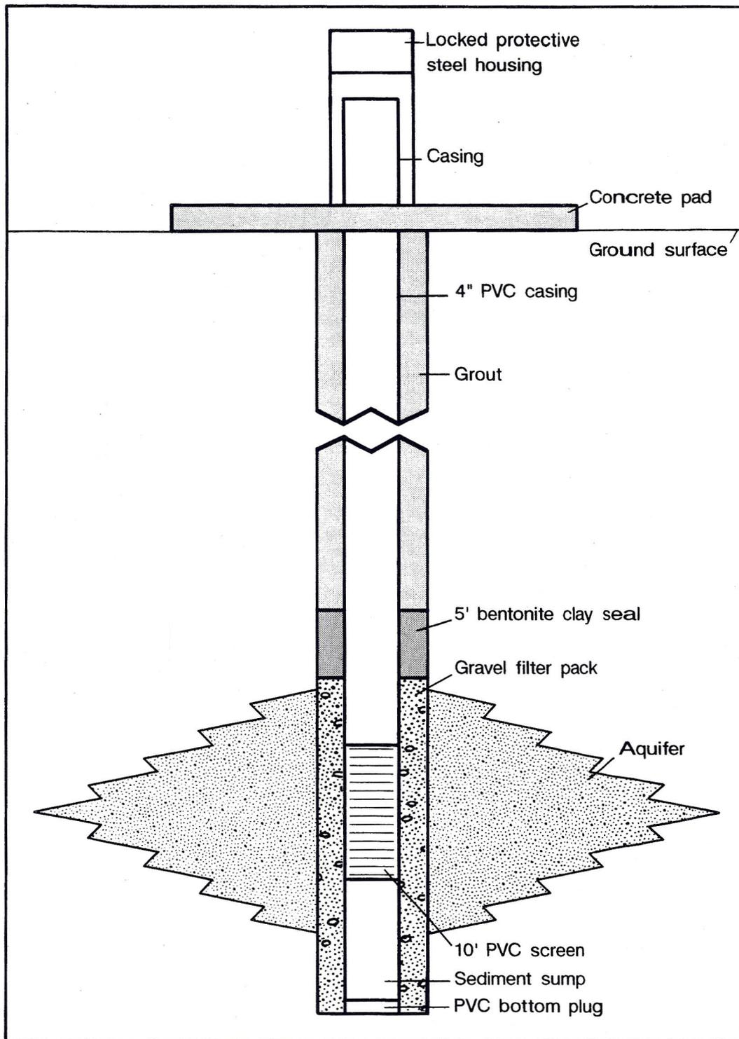
Figure 20. Details of a typical ground water monitoring well constructed for the Tritium Project.
