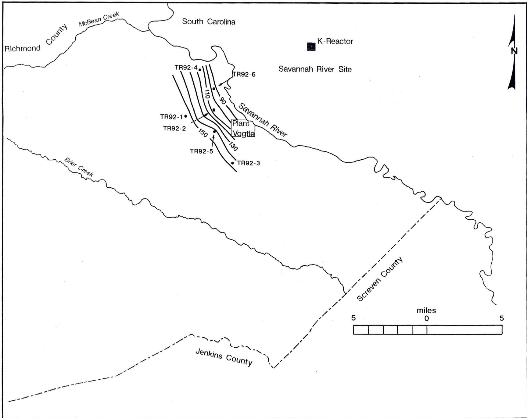
Figure 37. Local potentiometric surface map of the Gordon aquifer, as defined by data from Tritium Project monitoring wells. Elevations are in feet above mean sea level.
