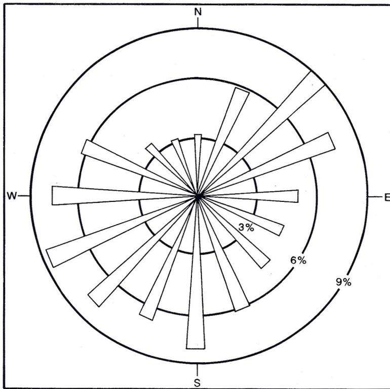
Figure 5. Wind rose plot (1987 - 1991) for the SRS-Burke County area, showing direction from which the wind blows and frequency of occurrence. (Modified from Aadland and others, 1993.)
