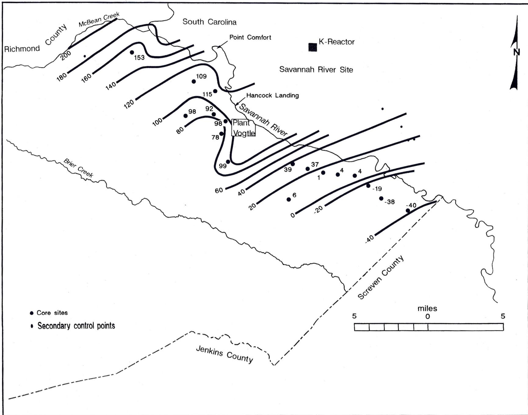
Figure 33. Structural contour map on the top of the Lisbon Formation. Elevations are in feet relative to mean sea level.
