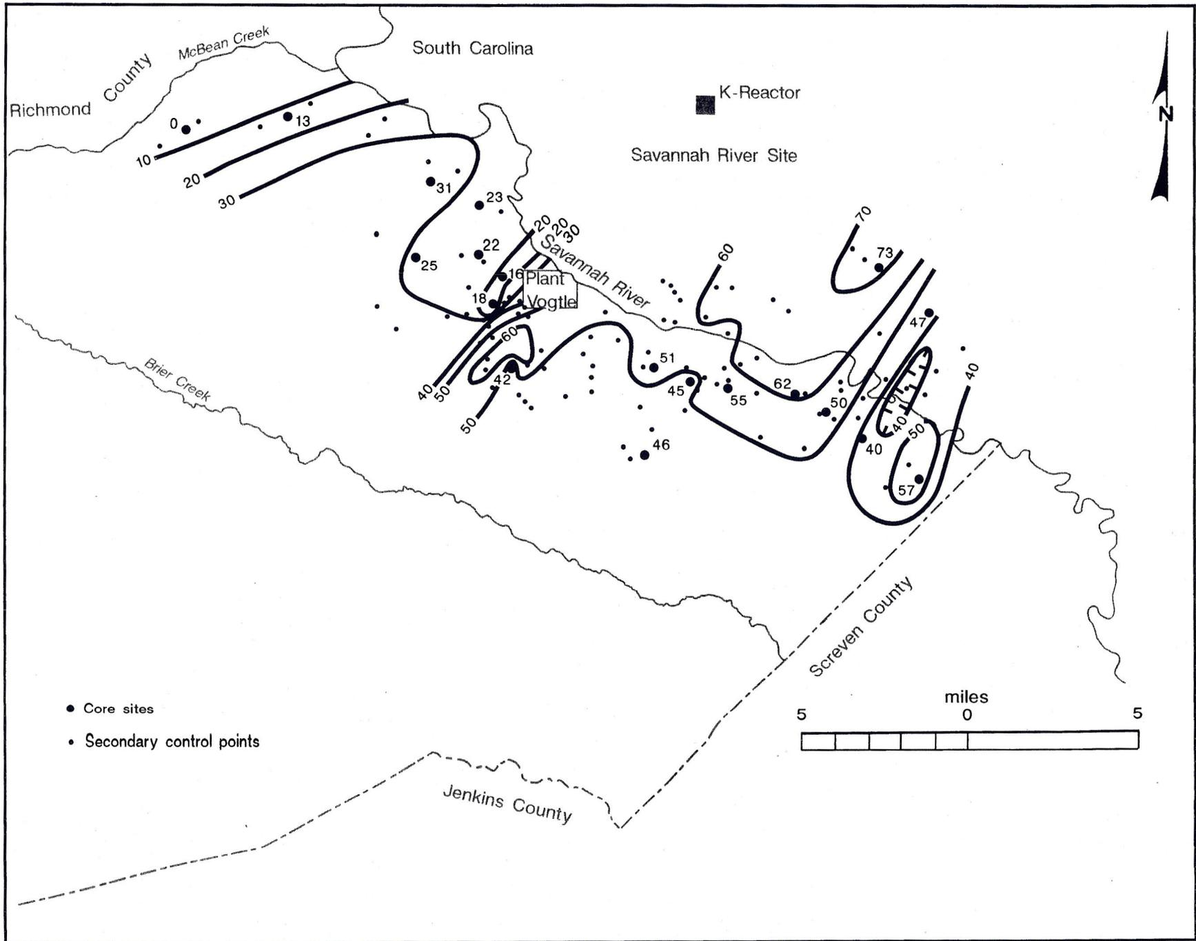
Figure 30. Isopach (thickness distribution) map of the Unnamed Congaree-equivalent sand. Thicknesses are in feet.
