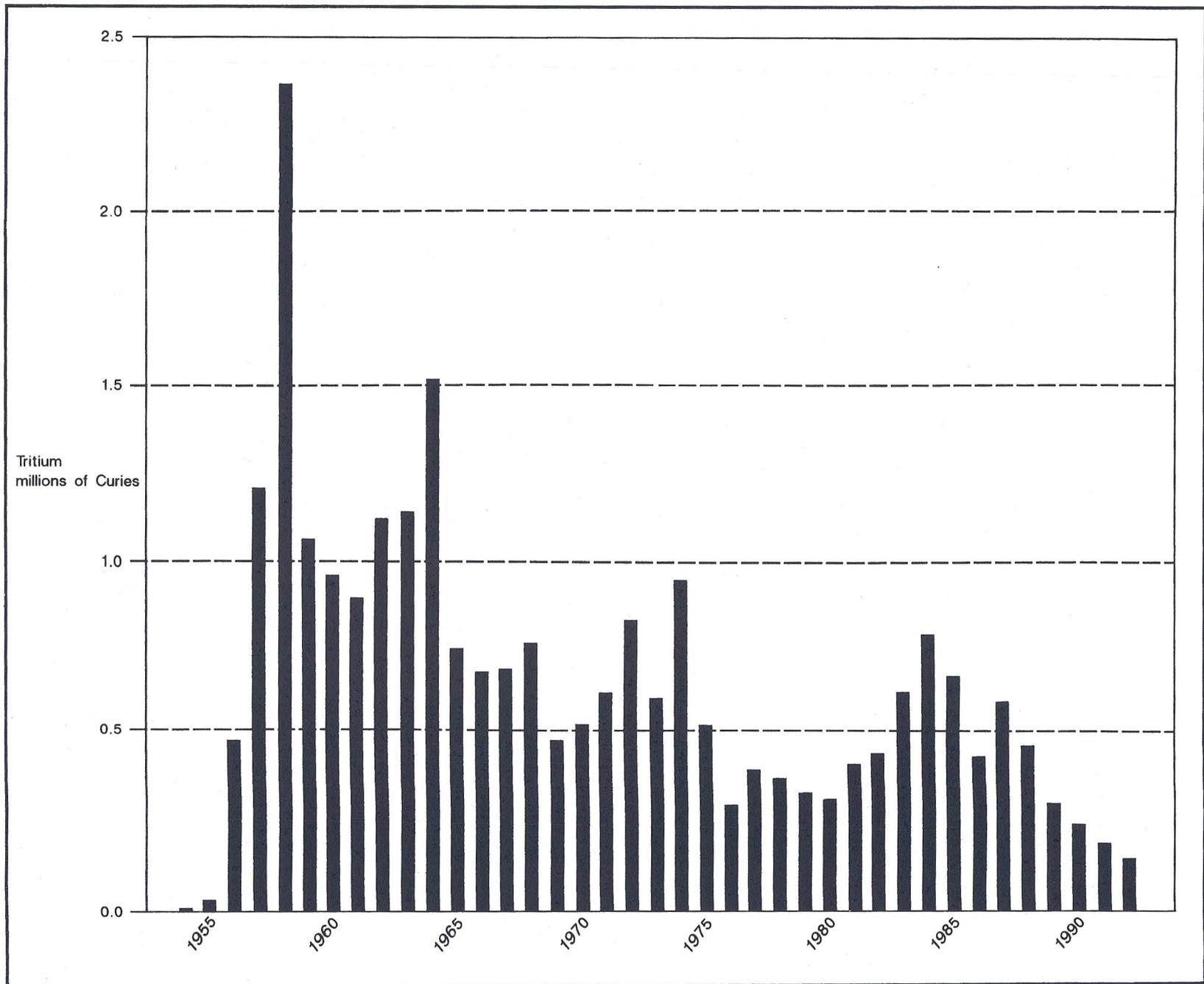
Figure 6. Bar graph showing comparisons of yearly SRS atmospheric tritium releases, 1954 - 1992. See Table 2 for sources. Values are not corrected for radioactive decay.
