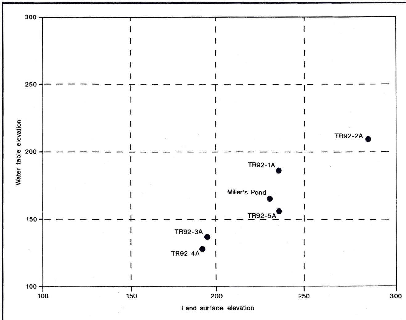
Figure 36. Relationship of water table and land surface elevations for the Upper Three Runs aquifer in eastern Burke County. Elevations are in feet above mean sea level.
