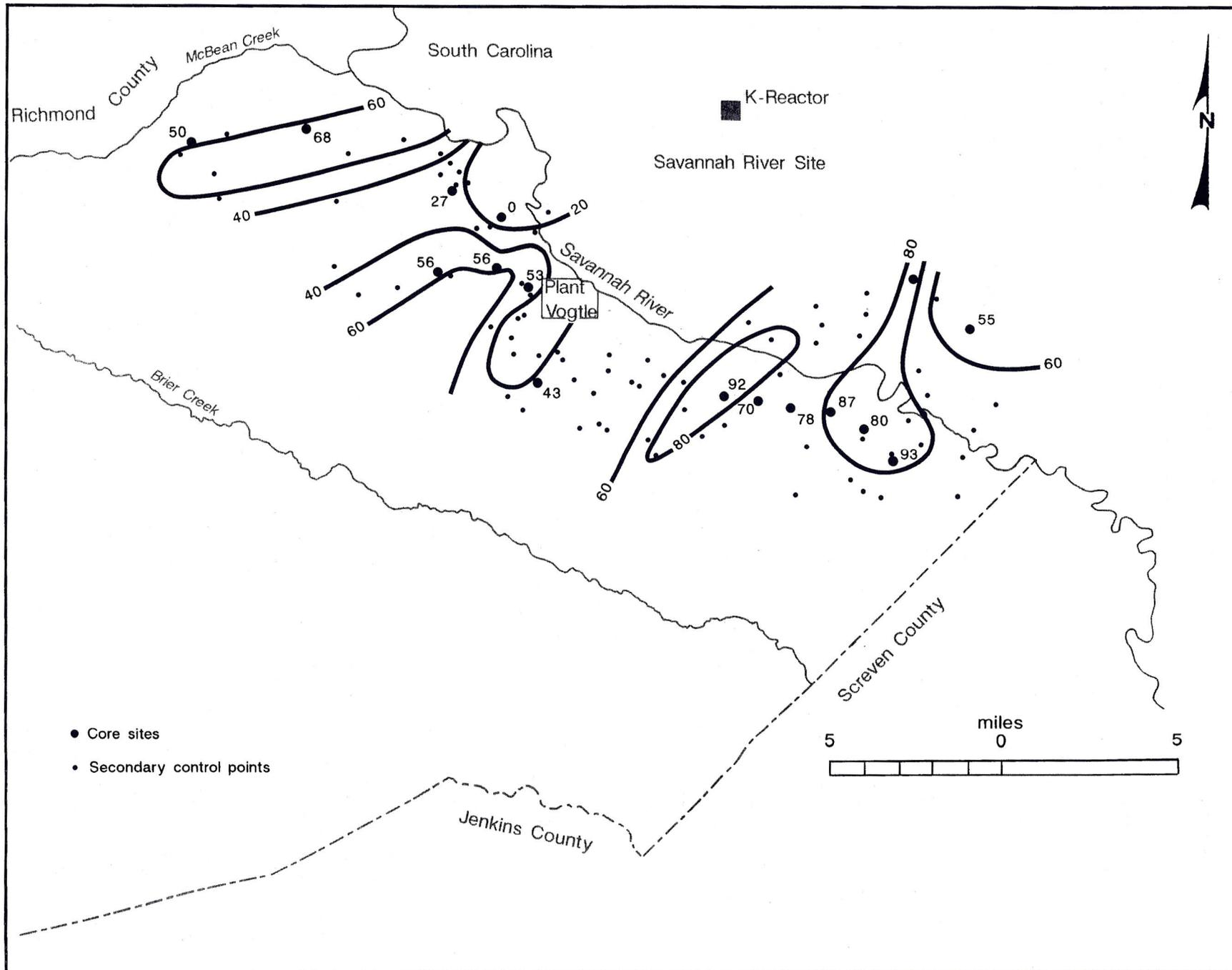
Figure 31. Isopach (thickness distribution) map of the Snapp Formation. Thicknesses are in feet.
