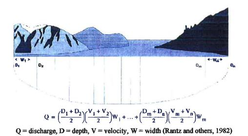
Figure 1. Stream cross section illustrating mid-section method to determine
