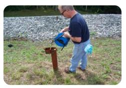
4. Record the depth from the top of the standing pipe (the established reference point) on the inspection sheet in the appropriate field. In addition, record the current lake water level.
