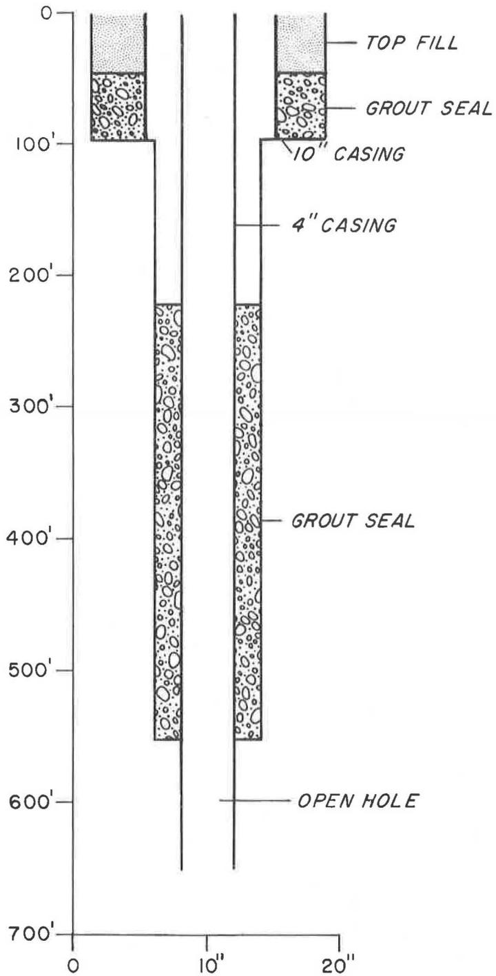
Figure B-2. Diagram of well construction for CI-01 (GGS 3426).
