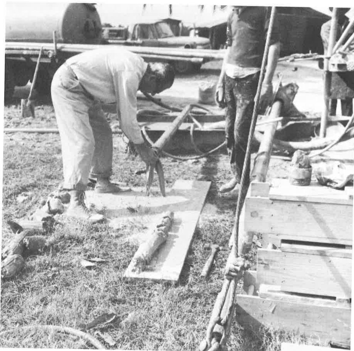
Figure 6. Removing core from barrel. Some core section on board. Outer core barrel, right center, attached to cable. Core boxes to right.
