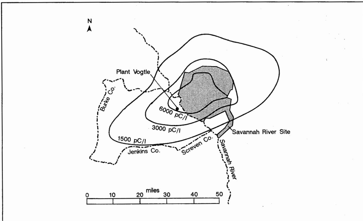
Figure 6. Directional distribution of tritium in rainfall for SRS-Burke County area, based on analyzed rainfall samples (1982-1986). Values are stated in picoCuries per liter. Modified from Murphy and others (1991).
