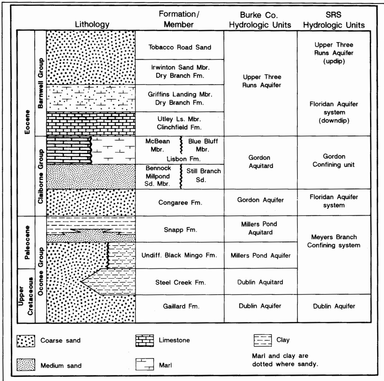
Figure 7. Tritium Project stratigraphic and hydrostratigraphic units for Burke County and the SRS area. Terminology from Aadland and others (1992), Falls and Baum (1995), Huddlestun and Summerour (1996), Falls and others (1997). Modified from Huddlestun and Summerour (1996).
