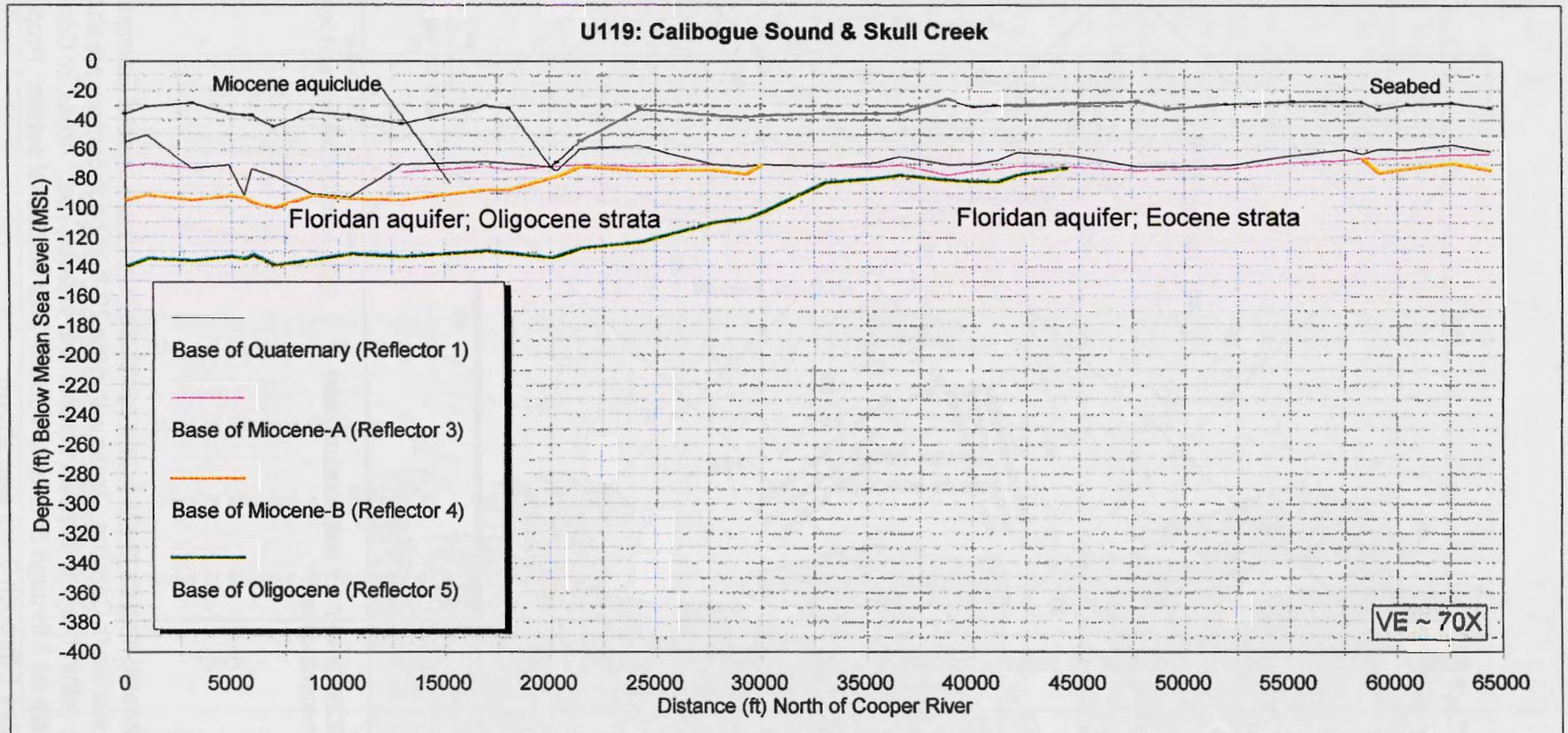
Figure 3-6 Coast-parallel oriented cross section from Skull Creek between Calibogue Sound and Port Royal Sound. Data-sample points are shown as black dots on the seabed reflector. Most of this section is contained within AOC #2. See Fig. 3-1 for location.
