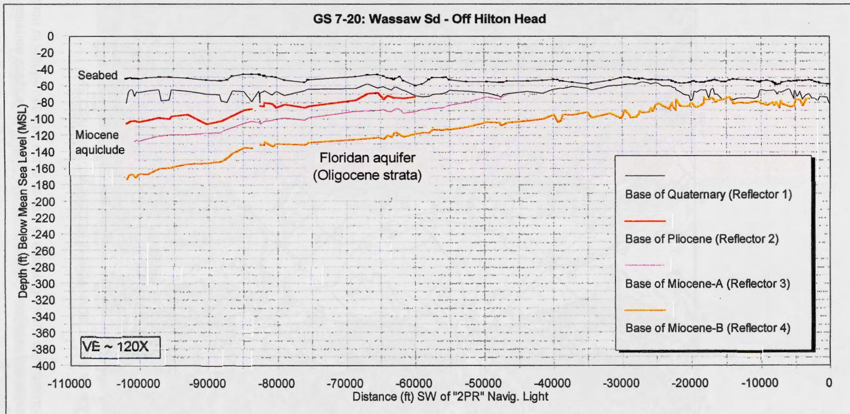
Figure 3-3 Coast-parallel oriented cross section along Seismic Line GS7-20 between offshore Tybee Island and offshore Hilton Head Island. Data-sample points are shown as black dots on the seabed reflector. AOC #1 occurs where Quaternary paleochannels cut down to the Floridan aquifer at the northeastern end of this section. See Fig. 3-1 for location.
