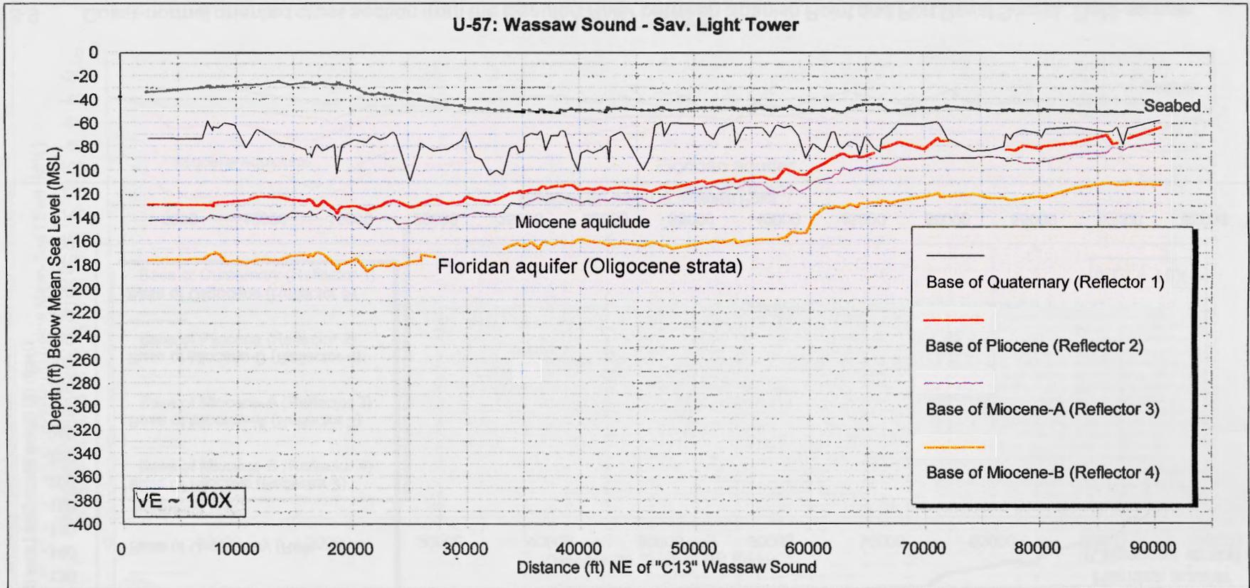
Figure 3-10 Coast-parallel oriented cross section along Seismic Line U-57 between Wassaw Sound and Savannah Light Tower. Data-sample points are shown as black dots on the seabed reflector. See Fig. 3-1 for location.
