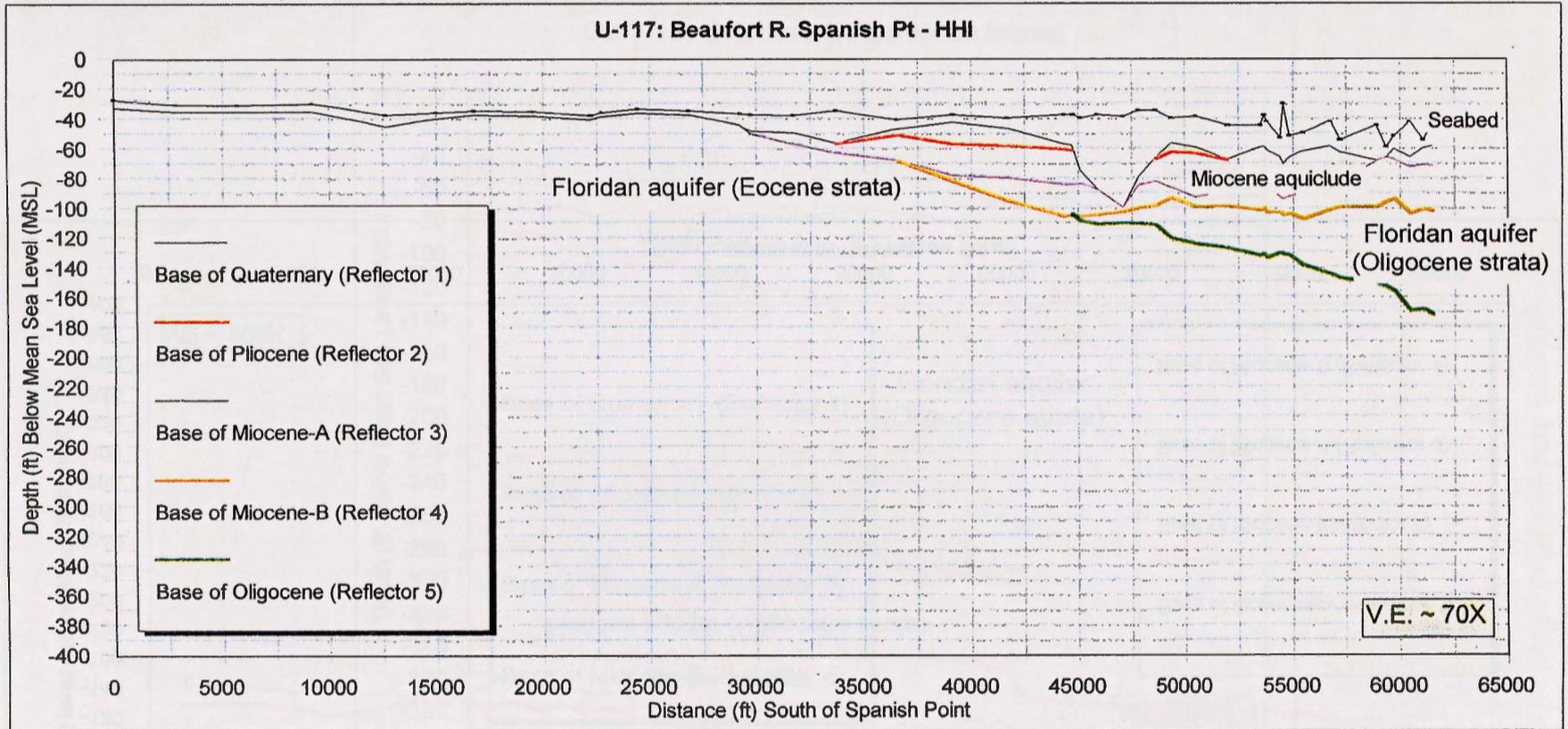
Figure 3-9 Coast-normal oriented cross section from the Beaufort River between Spanish Point and Port Royal Sound. Data-sample points are shown as black dots on the seabed reflector. AOC #5 encompasses the northern half of this section. See Fig. 3-1 for location.
