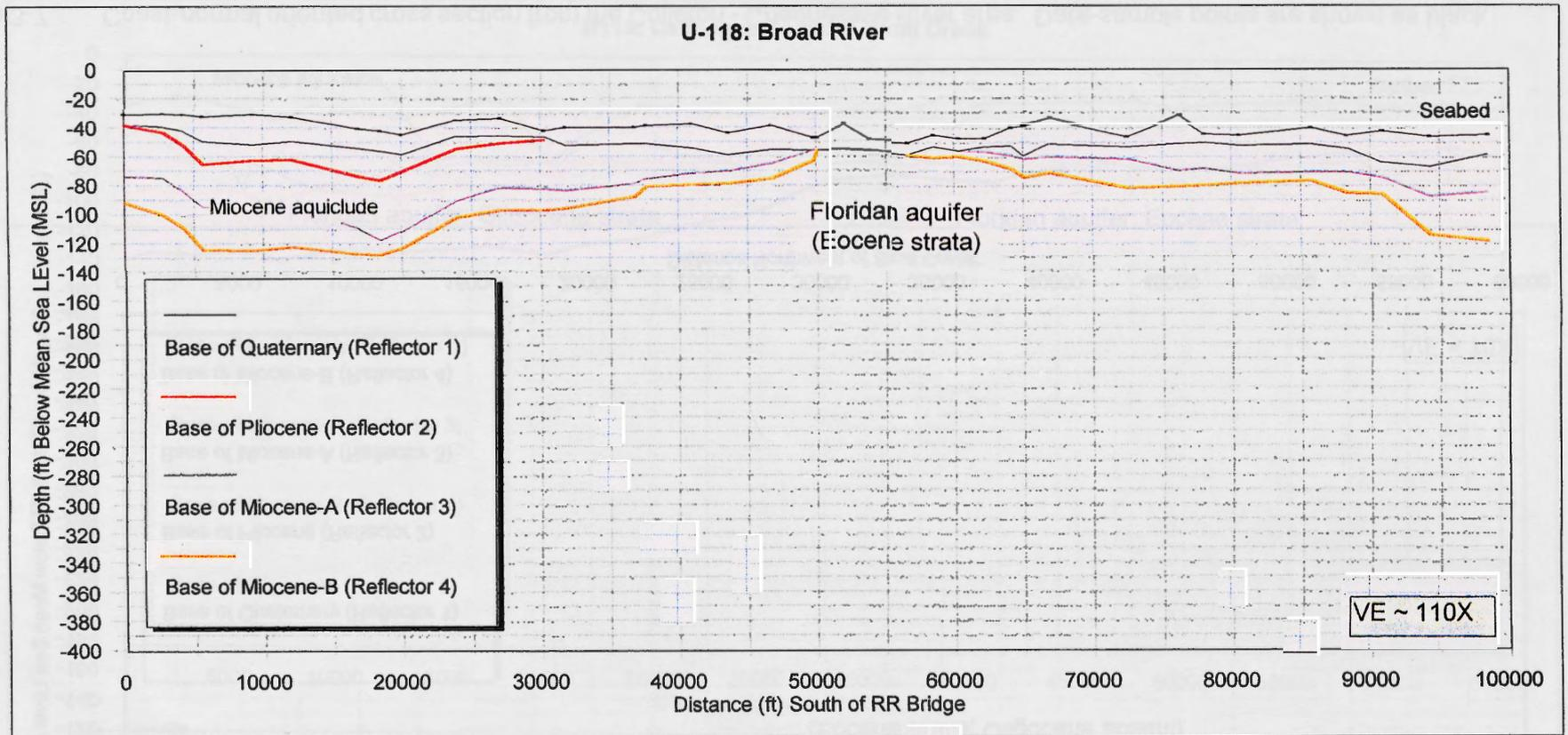
Figure 3-8 Coast-normal oriented cross section from the Broad River between Haulover Creek and Port Royal Sound. Data-sample points are shown as black dots on the seabed reflector. AOC #4 is centered on the aquifer high in the center of this section. See Fig. 3-1 for location.
