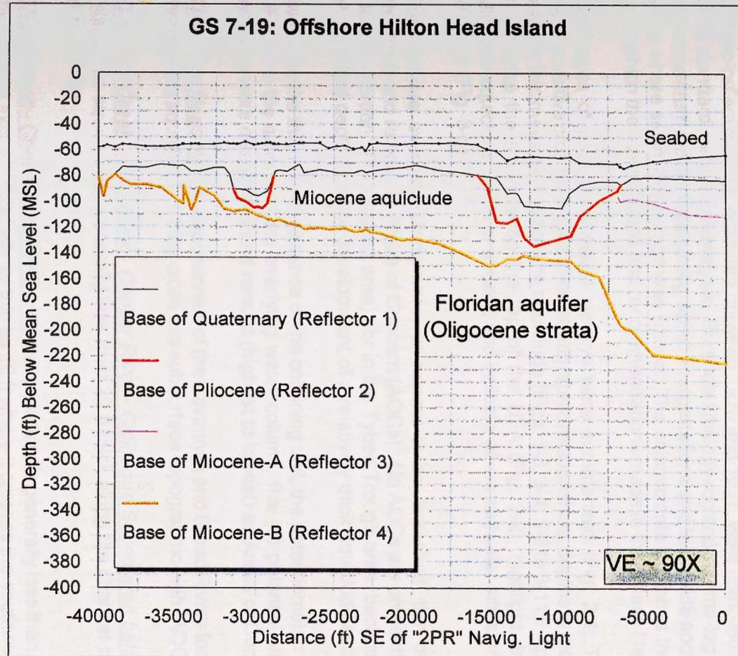
Figure 3-11 Coast-normal oriented cross section along Seismic Line GS7-19 offshore of Hilton Head Island. Data-sample points are shown as black dots on the seabed reflector. See Fig. 3-1 for location.
