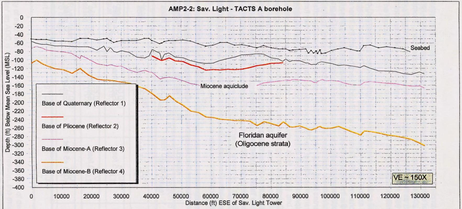
Figure 3-4 Coast-normal oriented cross section along Seismic Line AMP2-2 between Savannah Light Tower and the TACTS A borehole. Data-sample points are shown as black dots on the seabed reflector. See Fig. 3-1 for location.
