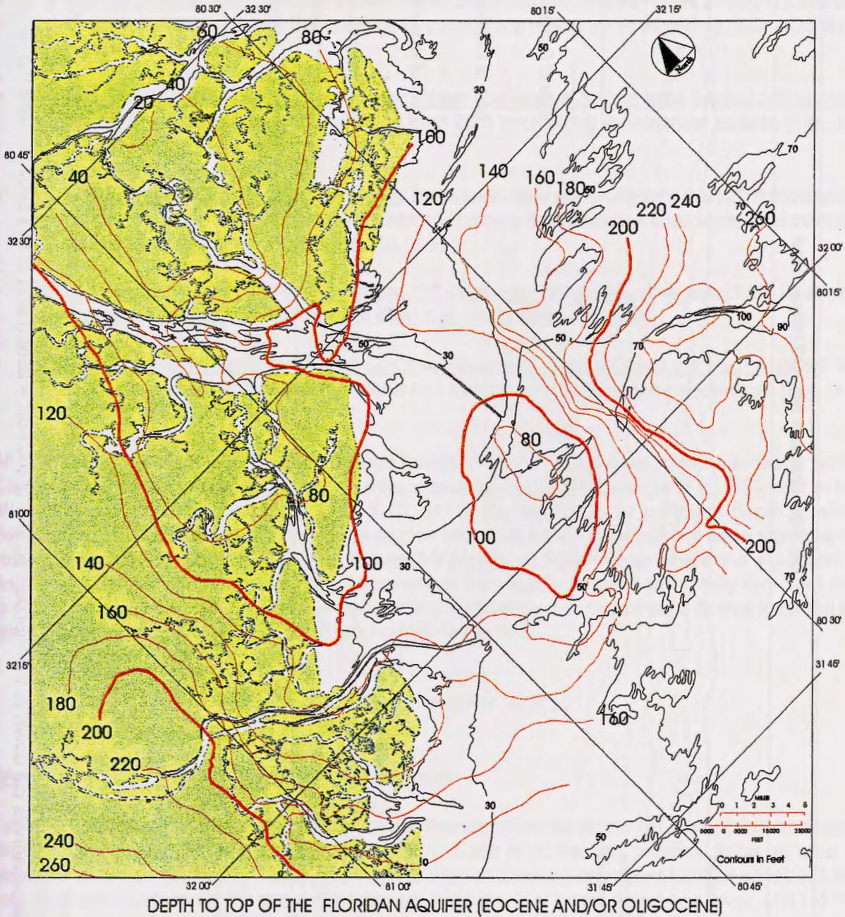
Figure 3-2 Structural contour map showing depths to the top of the Floridan aquifer in northern coastal Georgia and southern coastal South Carolina. This surface equates with seismic Reflector 4.
