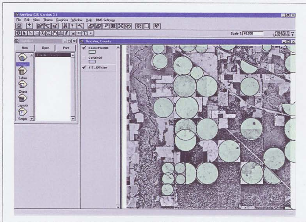
Figure 13. Center pivot irrigation sites were mapped in a heads-up digitizing environment using ArcView.
