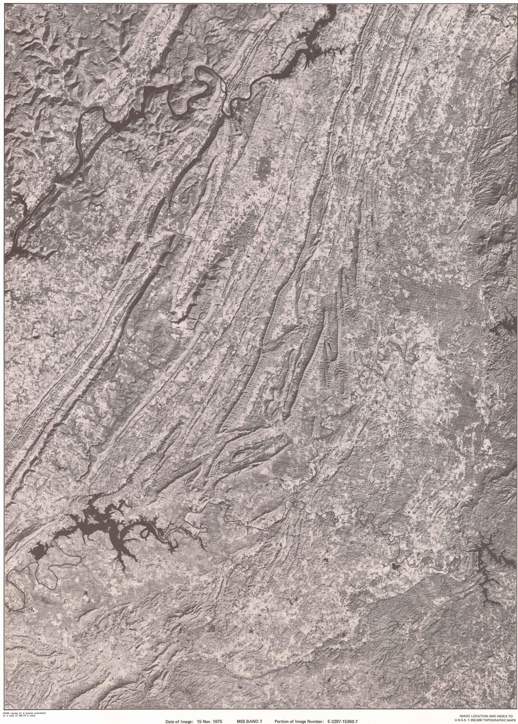
A band 7 infrared (800-1100 nm) satellite image from the National Aeronautics and Space Administration's Landsat (formerly ERTS) at an altitude of 567 miles (912 kilometers).
