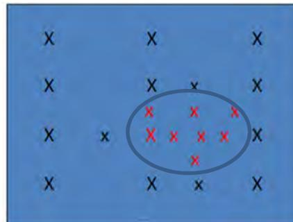
Phase 2 of Sampling: delineate hot spot using biased sampling. Sample locations are indicated by lowercase "x". Entire hot spot is represented by ellipse.
