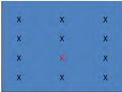
Phase 1 of Sampling: Use grid sampling to determine if there is any contamination within DU. One sample was identified as a hot spot. Implement Phase 2 sampling to delineate size of hot spot.
