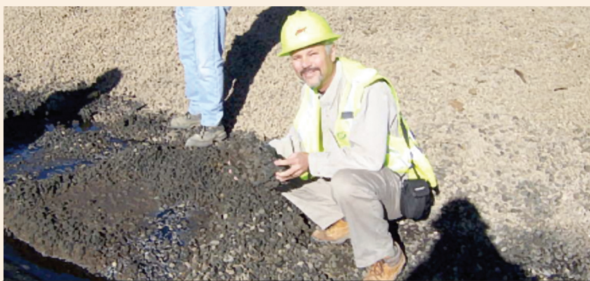
Photo 1. Author Richard Thiel holding 35 mm rounded gravel cemented by leachate chemical precipitation.
