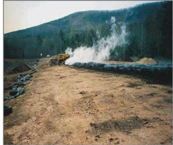
A composting system using large equipment to turn materials
