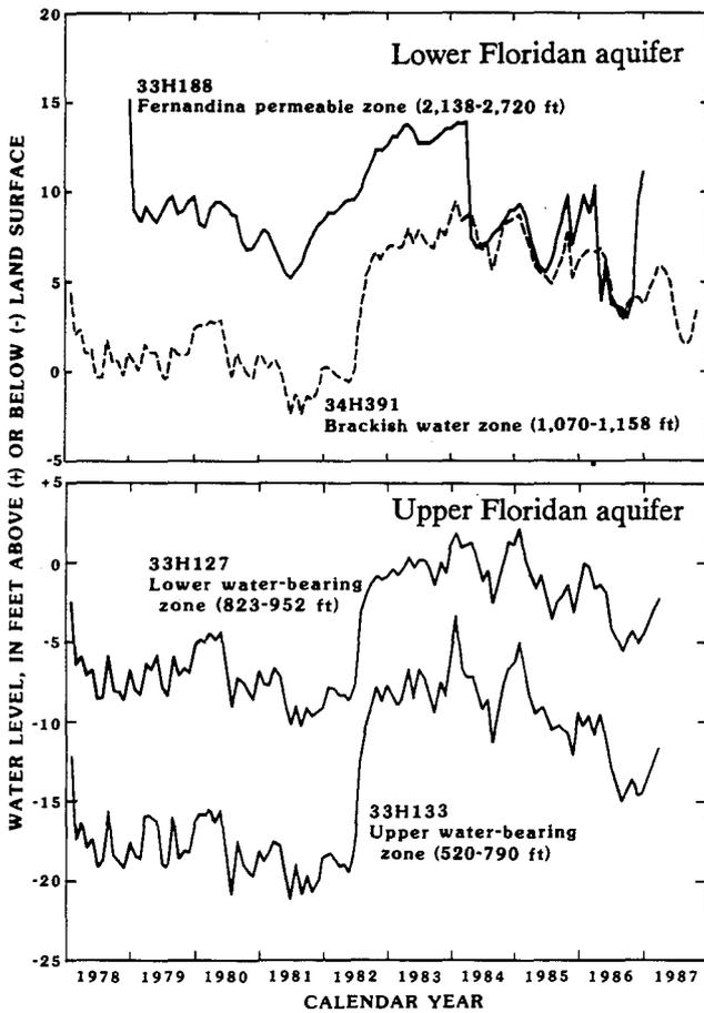
Figure 14.--Monthly mean water levels in the brackish-water zone and Fernandina permeable zone of the Lower Floridan aquifer, and in the upper and lower water-bearing zones of the Upper Floridan aquifer, Glynn County, 1978-87.
