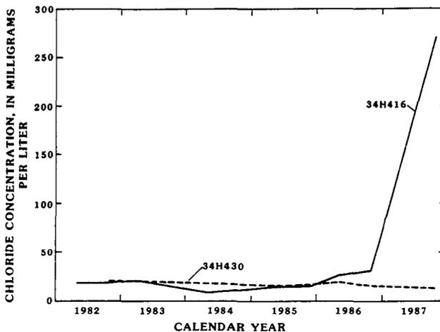
Figure 19.--Graph showing chloride concentration in the surficial aquifer at wells 34H416 and 34H430, Glynn County, 1982-87.
