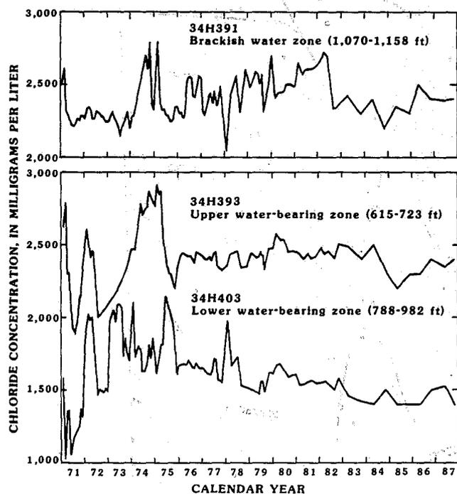
Figure 24.--Chloride concentration in the brackish-water zone of the Lower Floridan aquifer, and in the upper and lower water-bearing zones of the Upper Floridan aquifer in the Bay Street area of Brunswick, 1971-87.
