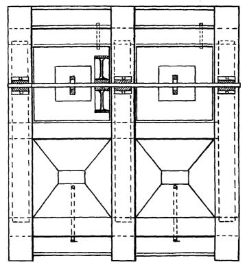
Fig. 25. Plan of 2-cell jig, showing arrangement of plunger and screen cells, position of drive shaft and eccentrics.
