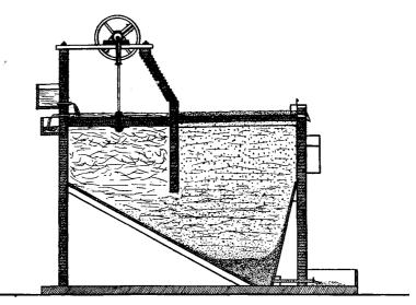
Fig. 26. Vertical cross section showing in a graphical way the action of a Harz jig.
