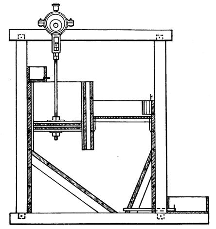
Fig. 24. Transverse section through jig box showing position of plunger and screen.
