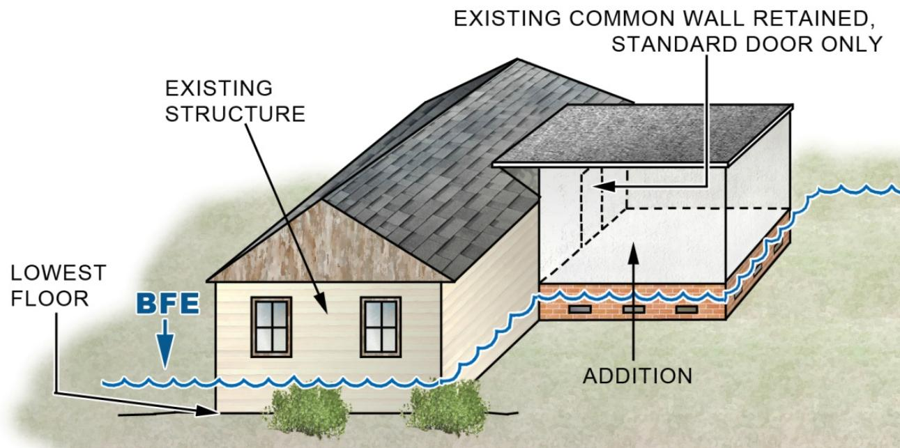
Figure 48. Substantial Improvement – Lateral Addition
