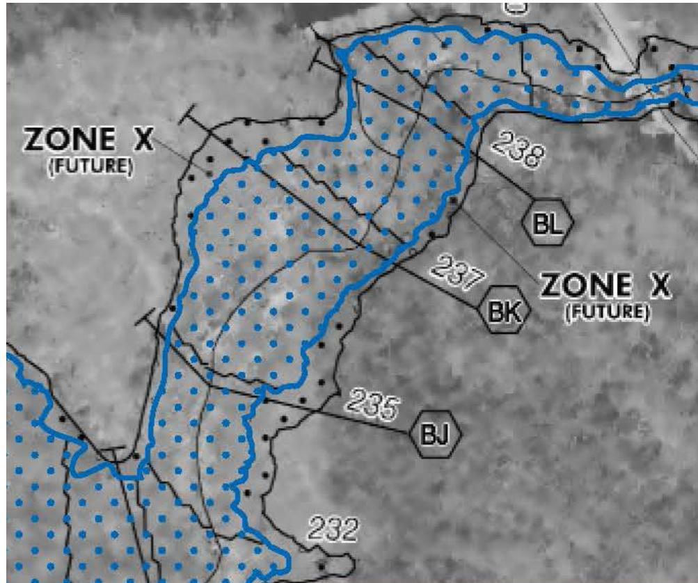
Figure 10. Future-condition floodplains on a FIRM
