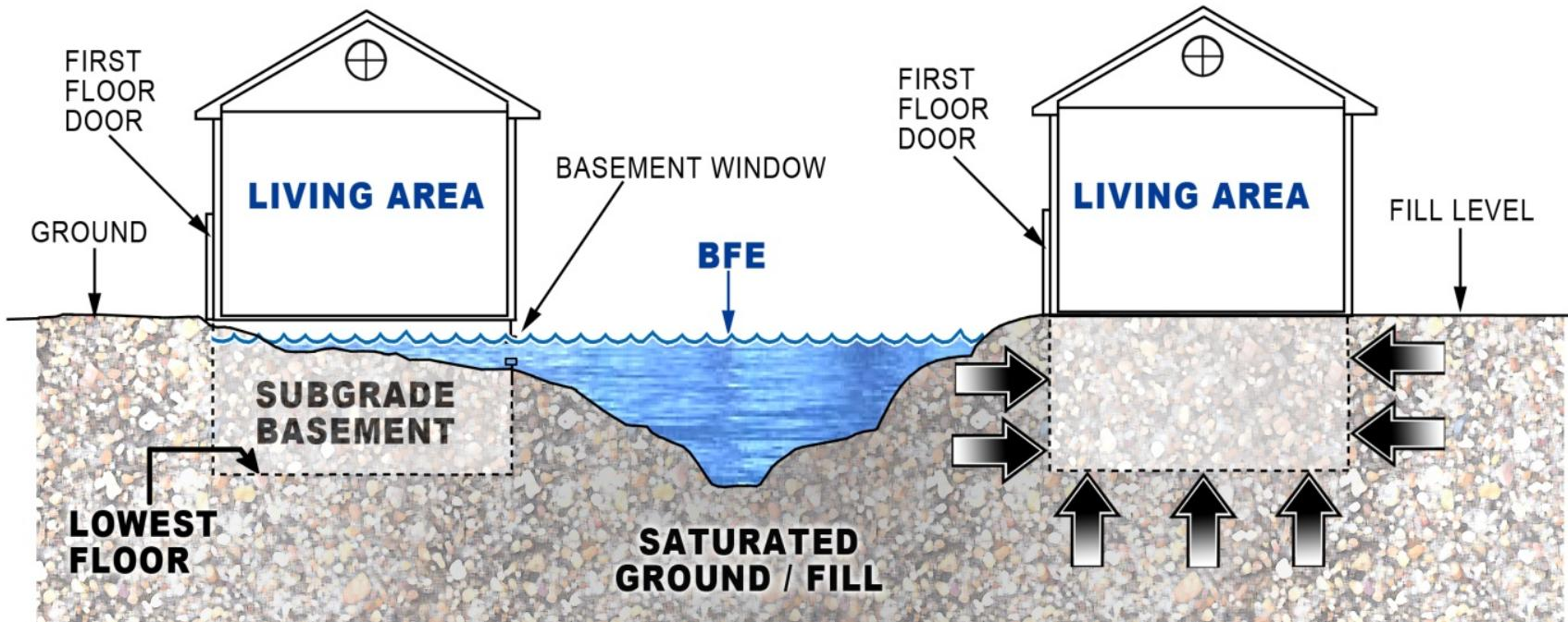
Figure 36. Basements are not allowed in new buildings in the SFHA
