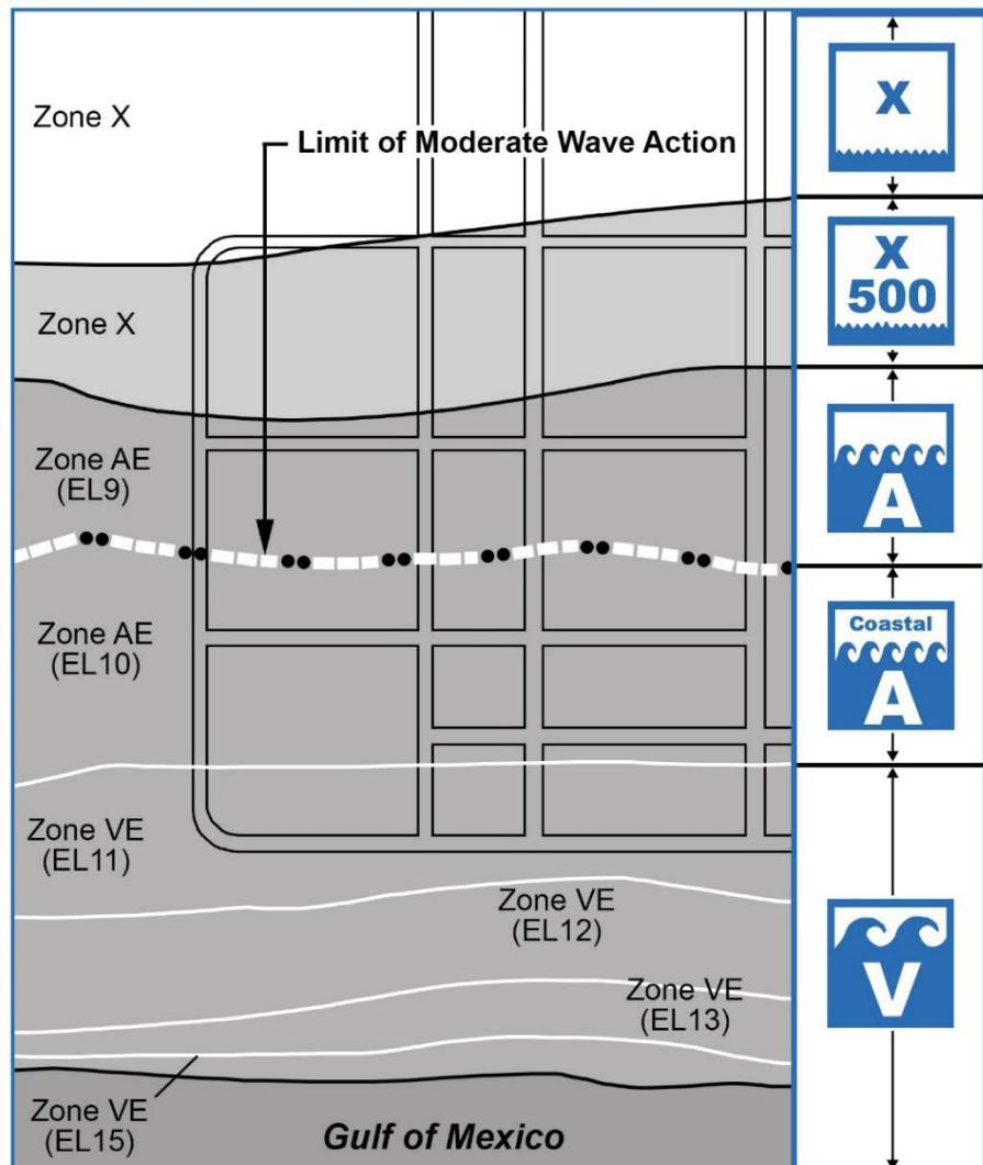
Figure 16. Example of a LiMWA on a FIRM
