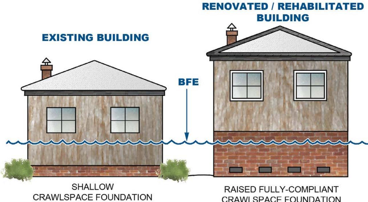
Figure 47. Substantially Improvement- Reconstruction on Existing Foundation
