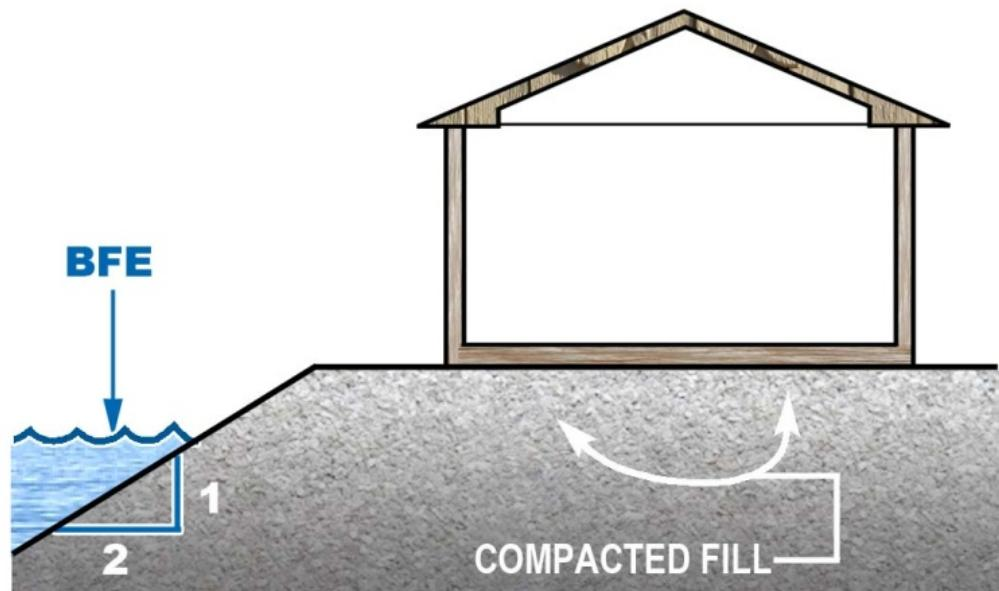
Figure 32.Fill Compaction and Slope Criteria
