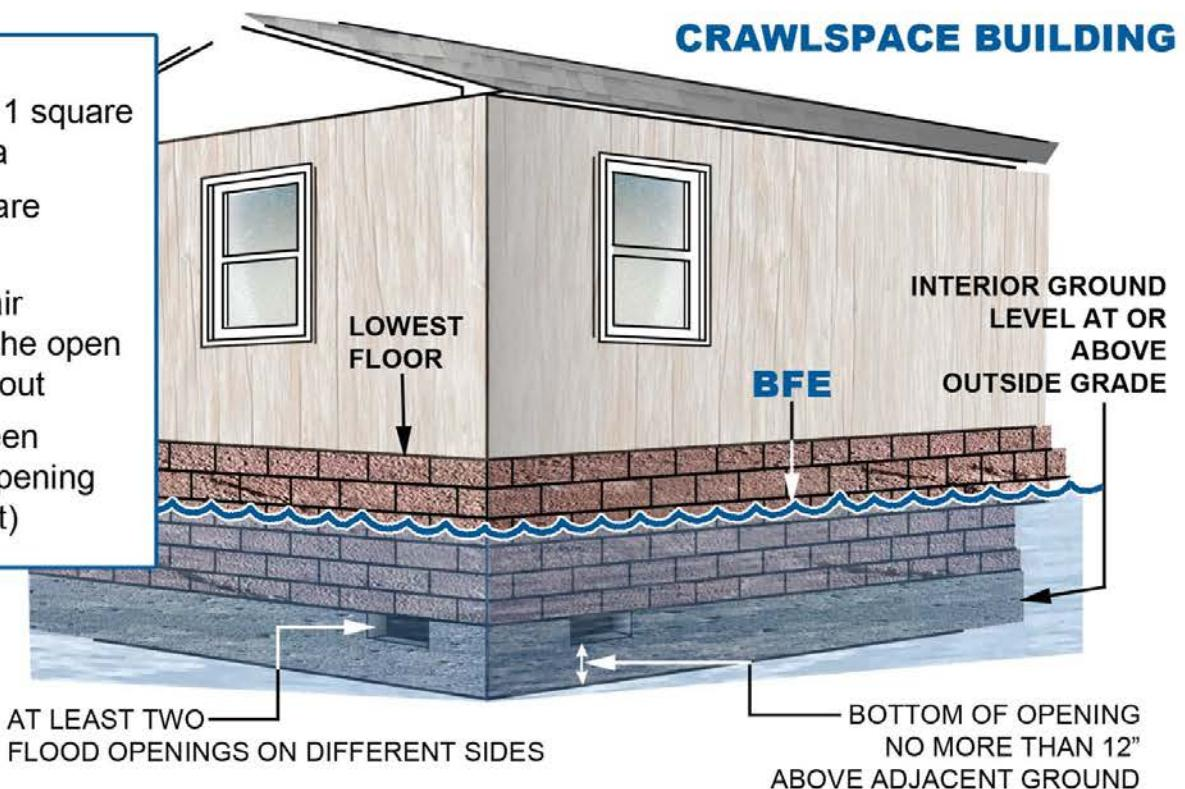
Figure 34. Flood Openings
