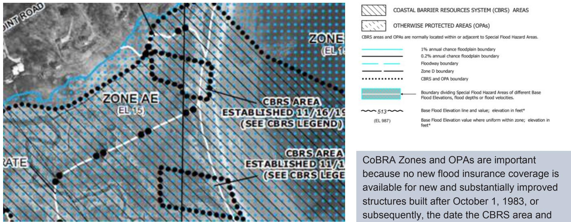
Figure 17. Coastal Barrier Resources System areas on a FIRM
