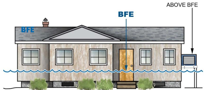
Figure 46. Example of a Low Cost Flood Protection Measure
