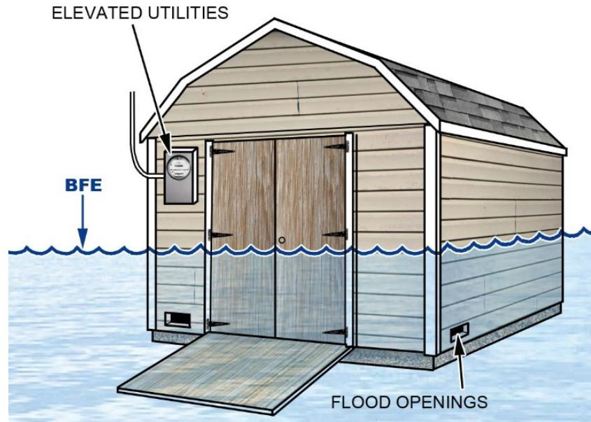
Figure 45. Accessory structure with flood openings and utilities elevated above the BFE
