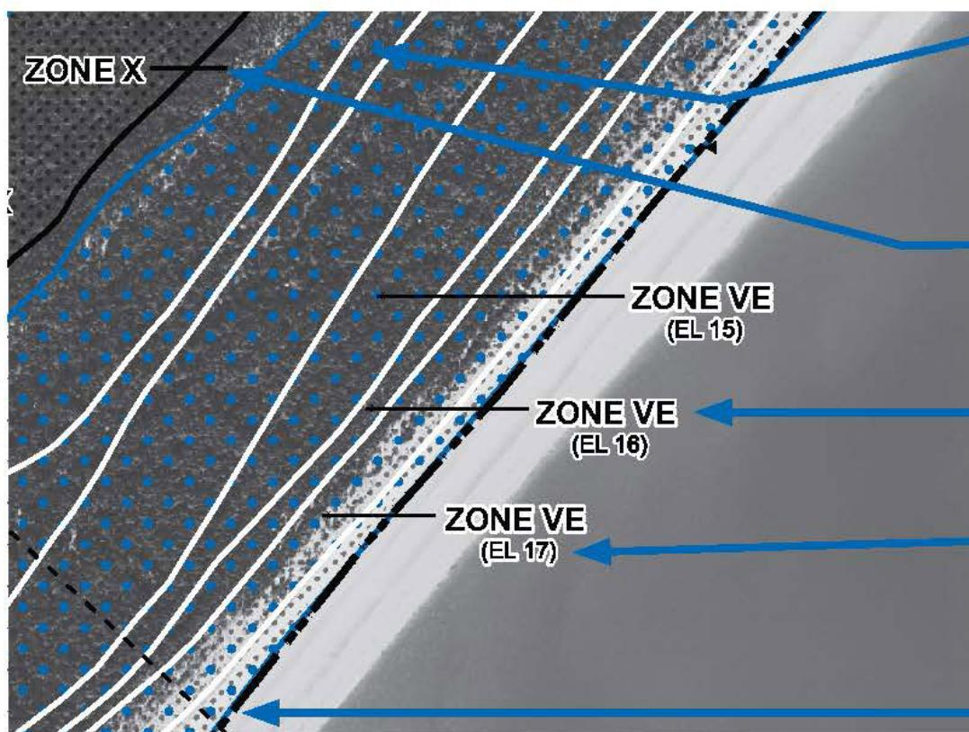
Figure 15. Coastal Flood Zones on a FIRM
