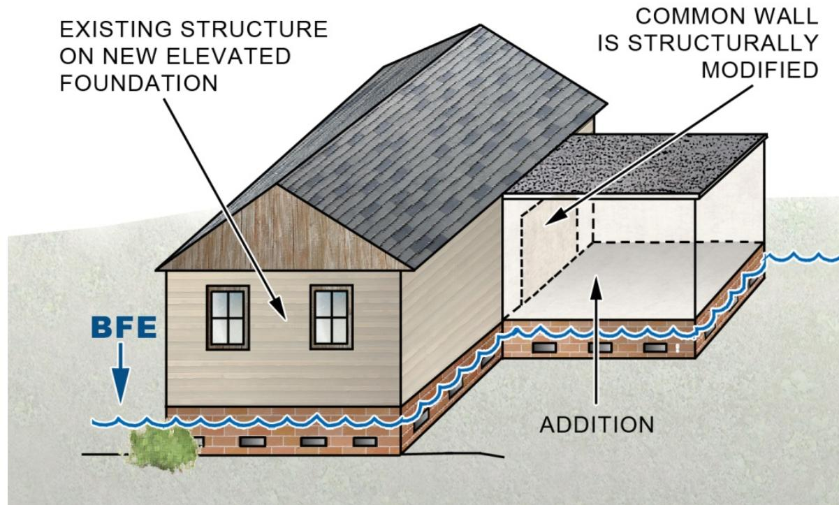
Figure 49. Substantial Improvement – Addition plus Other Work
