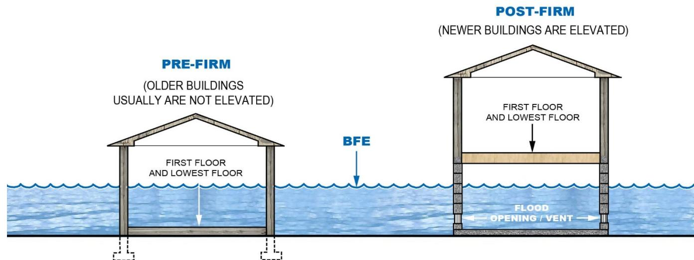
Figure 3. Pre-FIRM versus Post-FIRM construction
