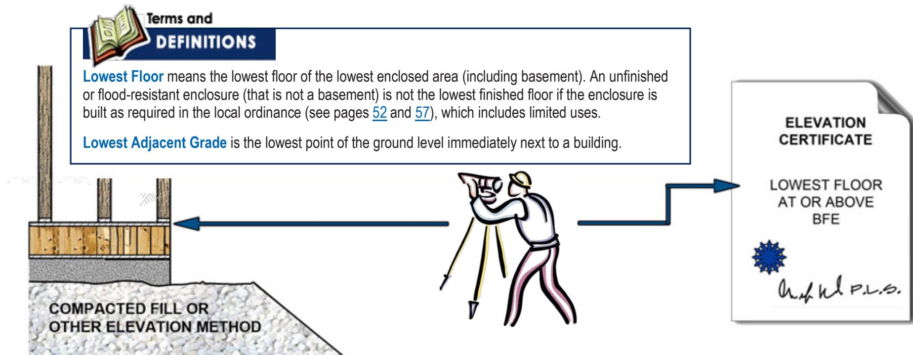
Figure 29. Survey Point of Lowest Floor
