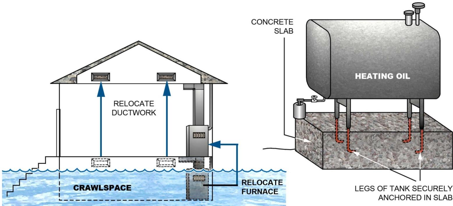
Figure 53. Low Cost Flood Protection Measures for Older Homes
