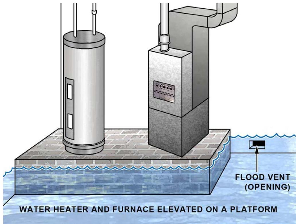
Figure 44. Utilities elevated on a platform
