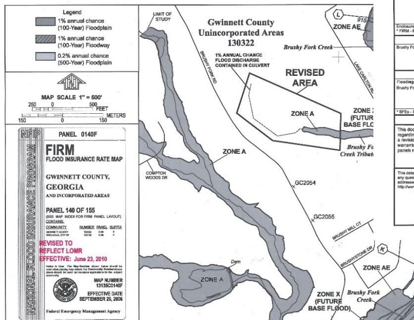
Figure 23. Example of a LOMR Determination Document
