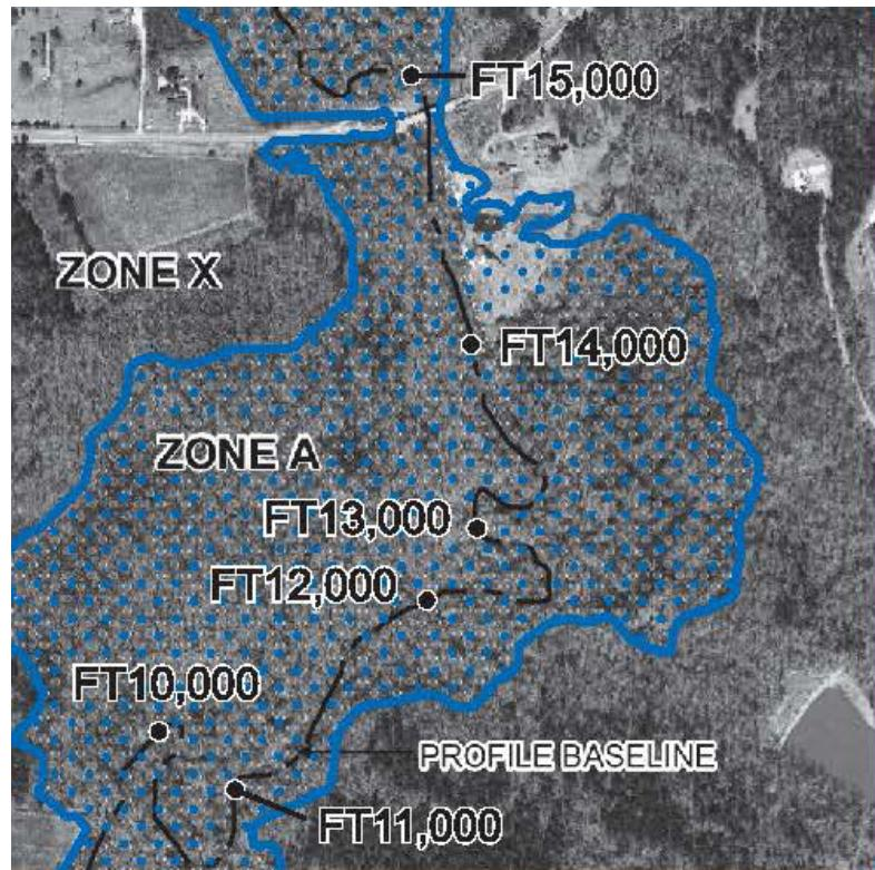
Figure 9. Limited Detailed Study on a FIRM
