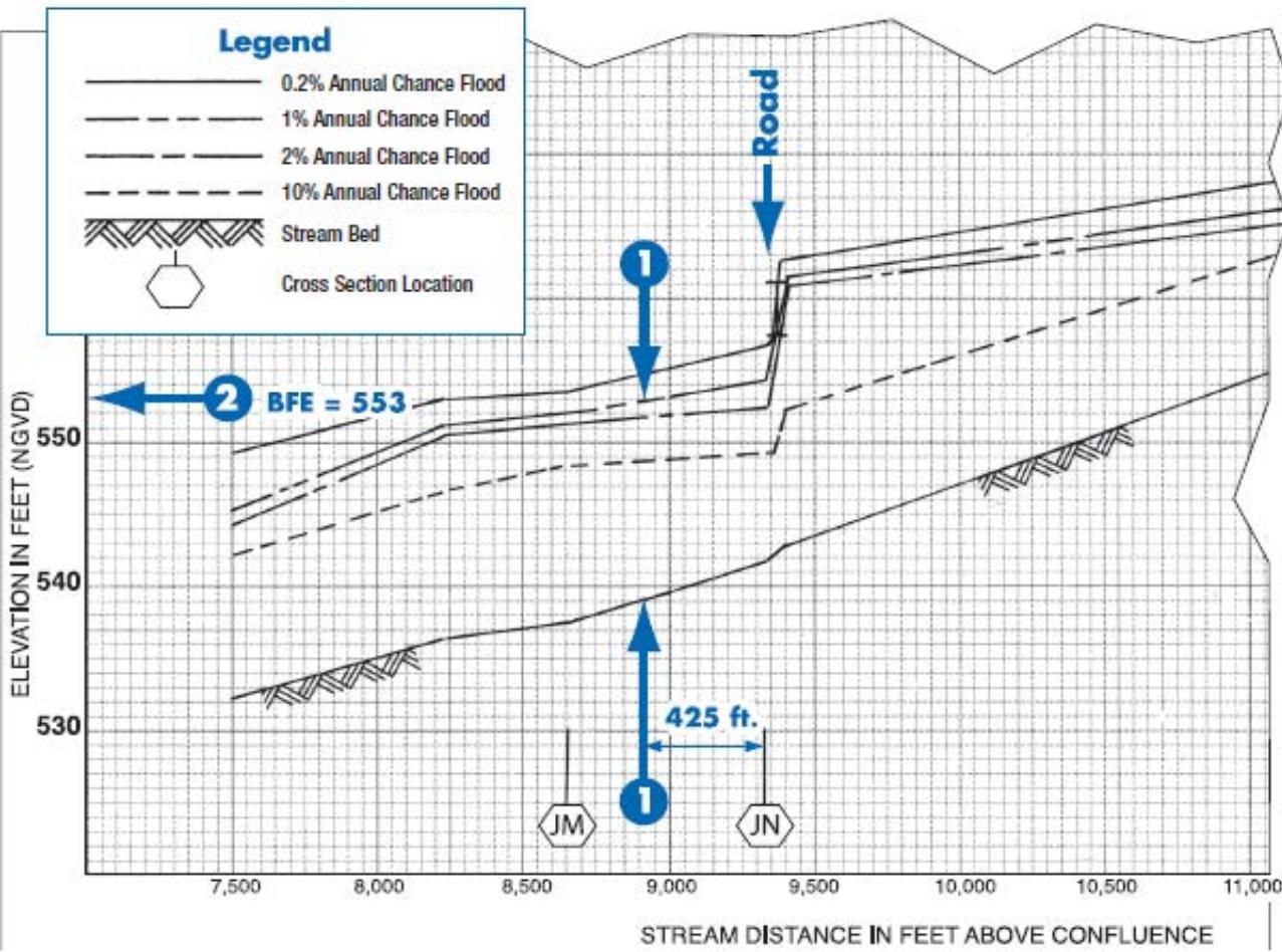
Figure 12. Flood Profile from an FIS Report
