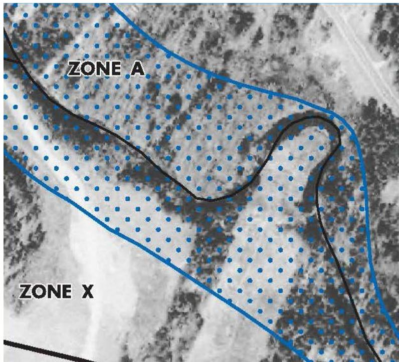
Figure 8. Approximate flood zone on a FIRM
