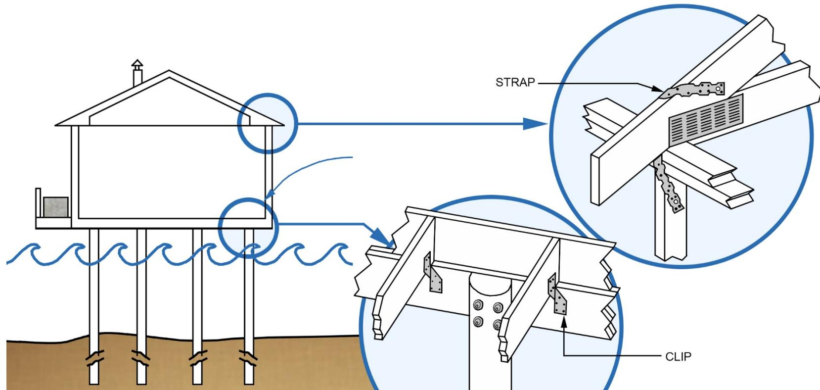
Figure 39. Wind Resistant Coastal Construction
