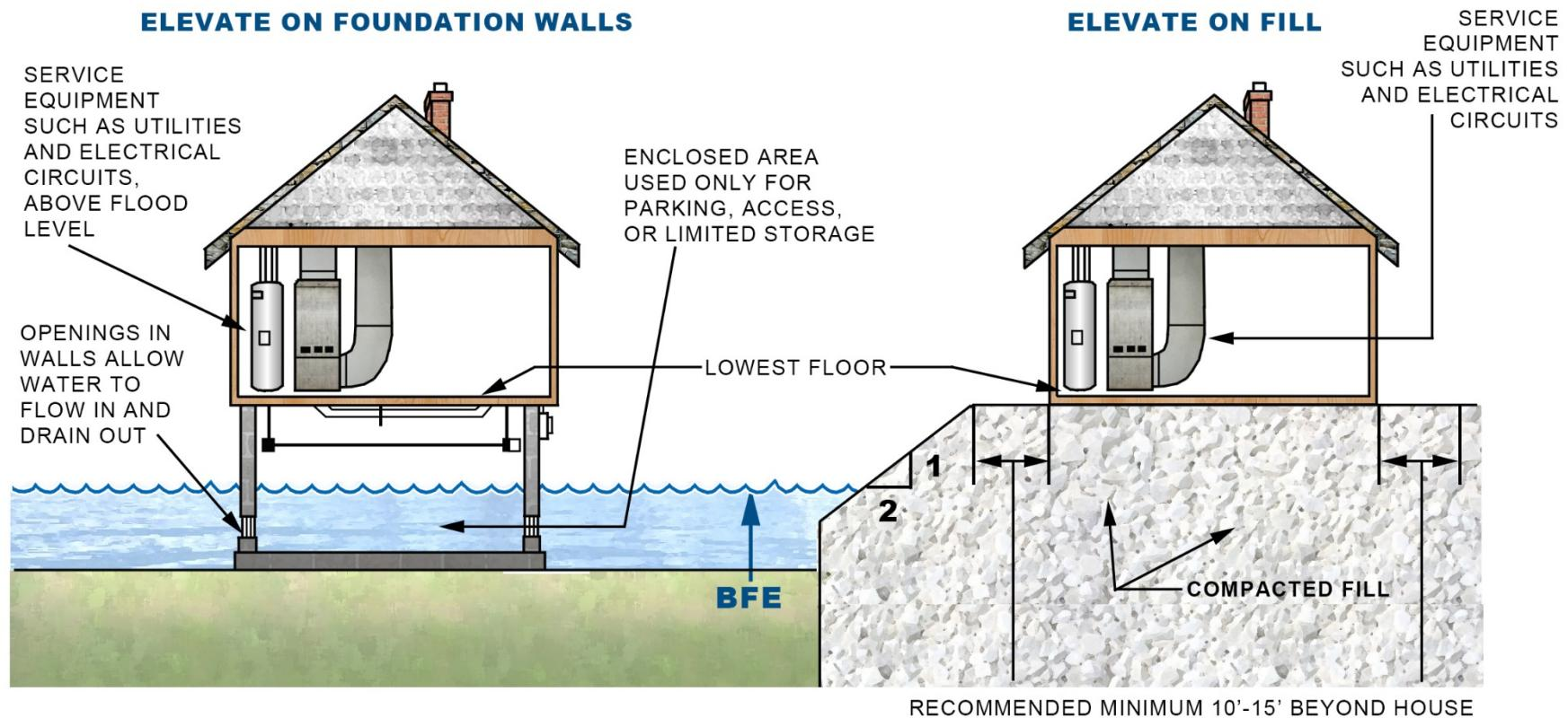
Figure 33.Elevation of Utilities
