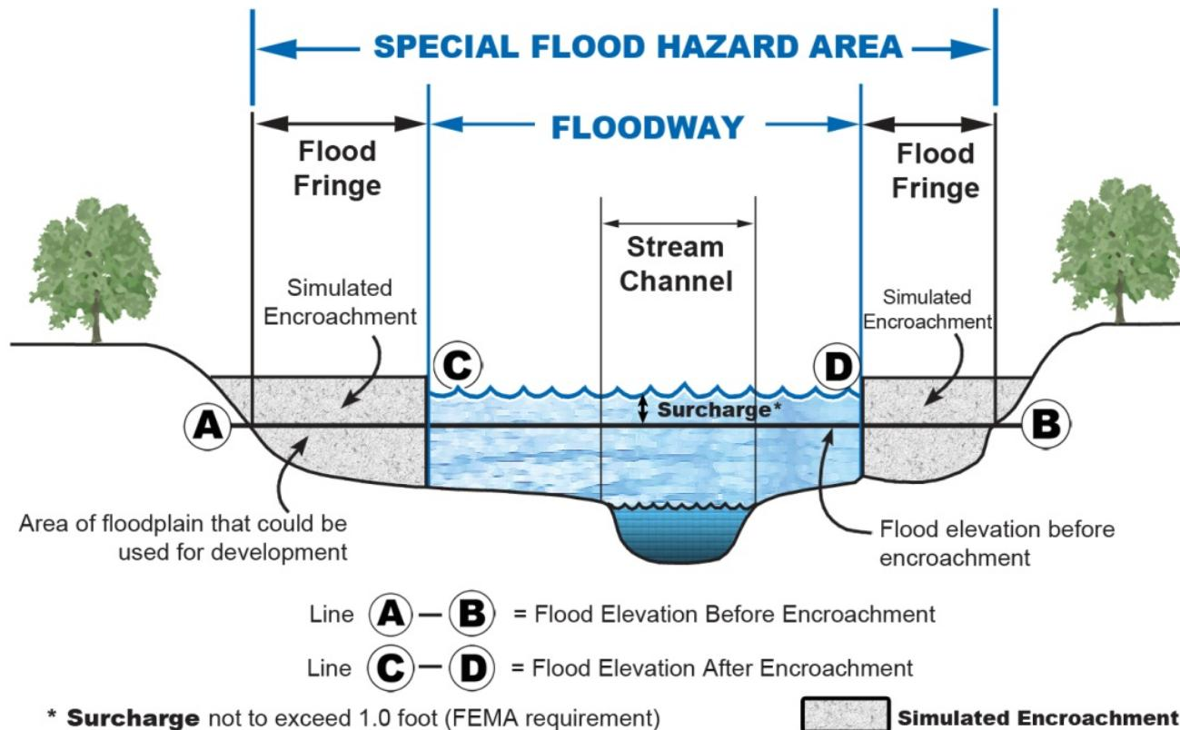
Figure 7. Floodway Schematic
