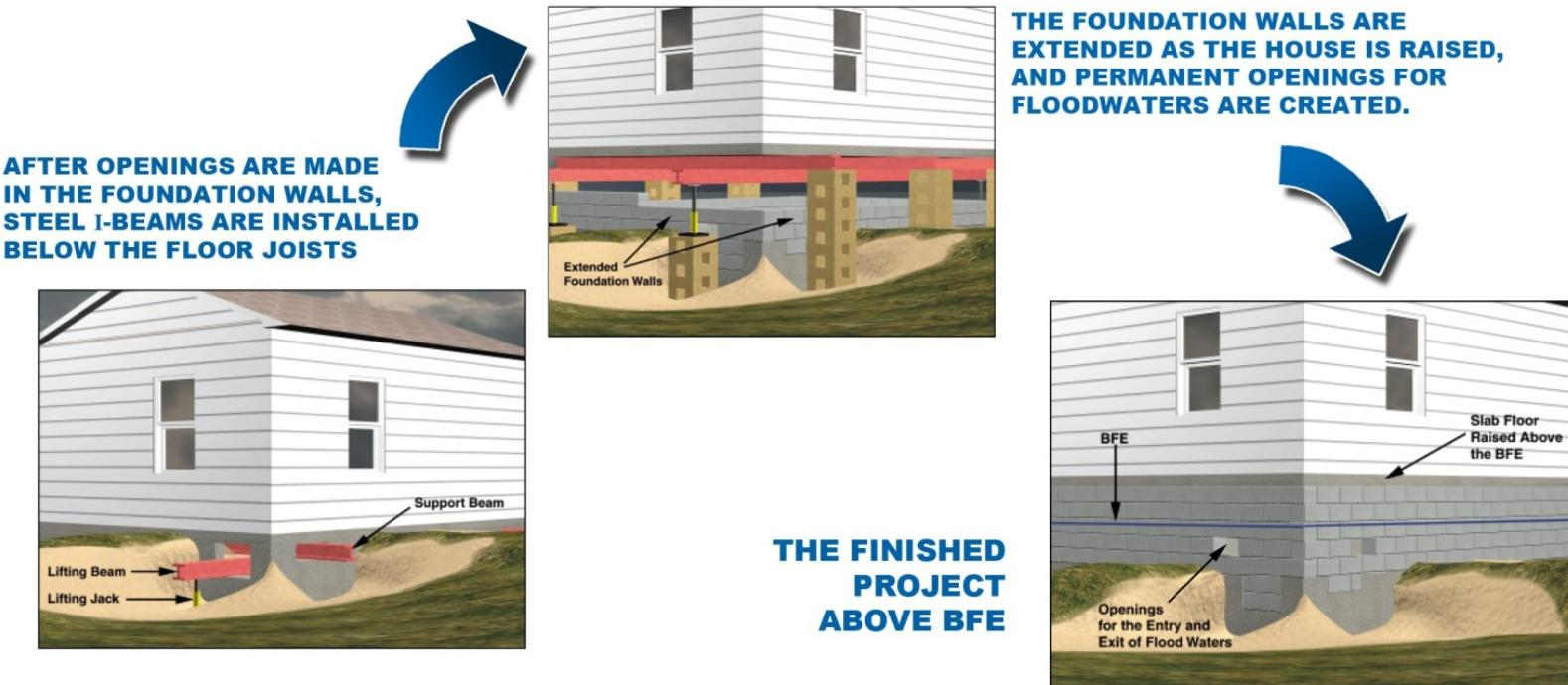
Figure 52. Elevating an Existing Building
