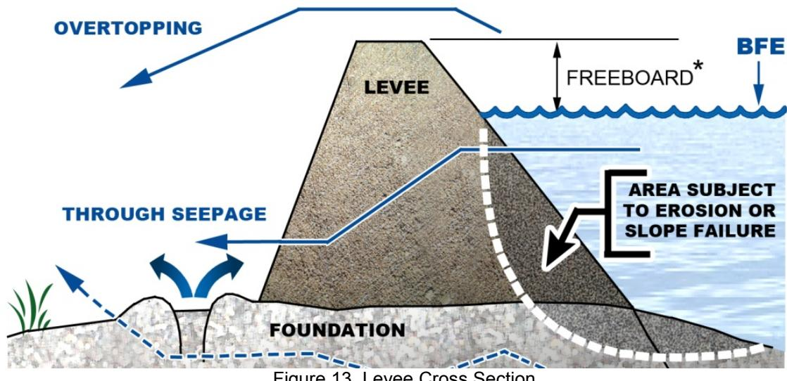
Figure 13. Levee Cross Section
