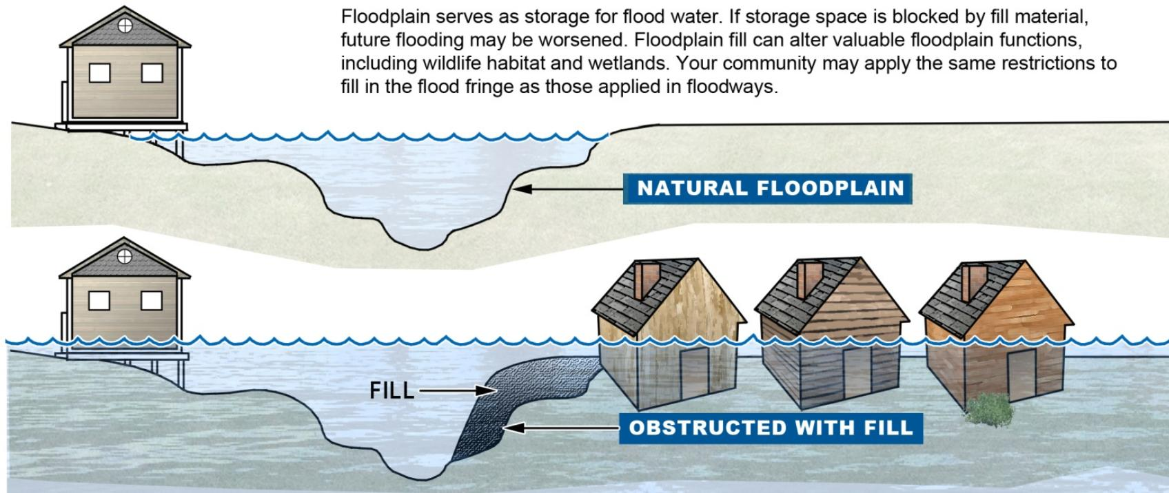
Figure 30. Obstructions Caused by Floodplain Fill
