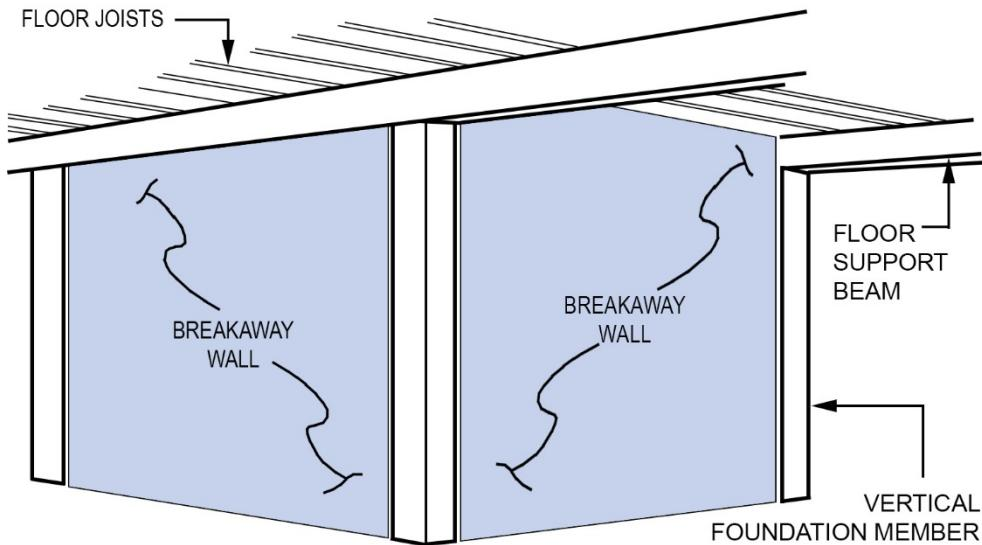
Figure 40. V Zone Construction Requirements
