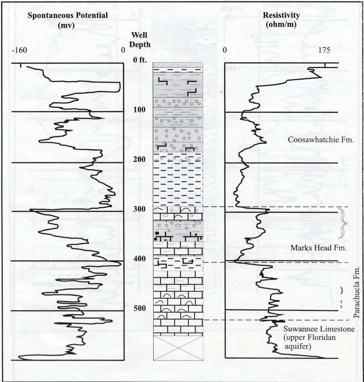
Figure 10: Stratigraphic column and electric logs of well 33K026, McIntosh County.
