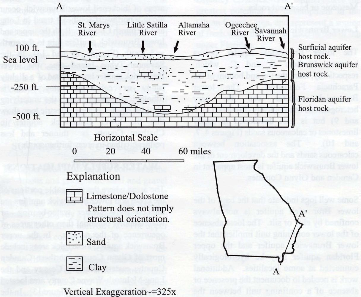
Figure 19: Generalized cross section showing stratigraphic relationship of shallow aquifers and the Floridan aquifer (modified from Watson, 1979). Depositional dips are not shown.
