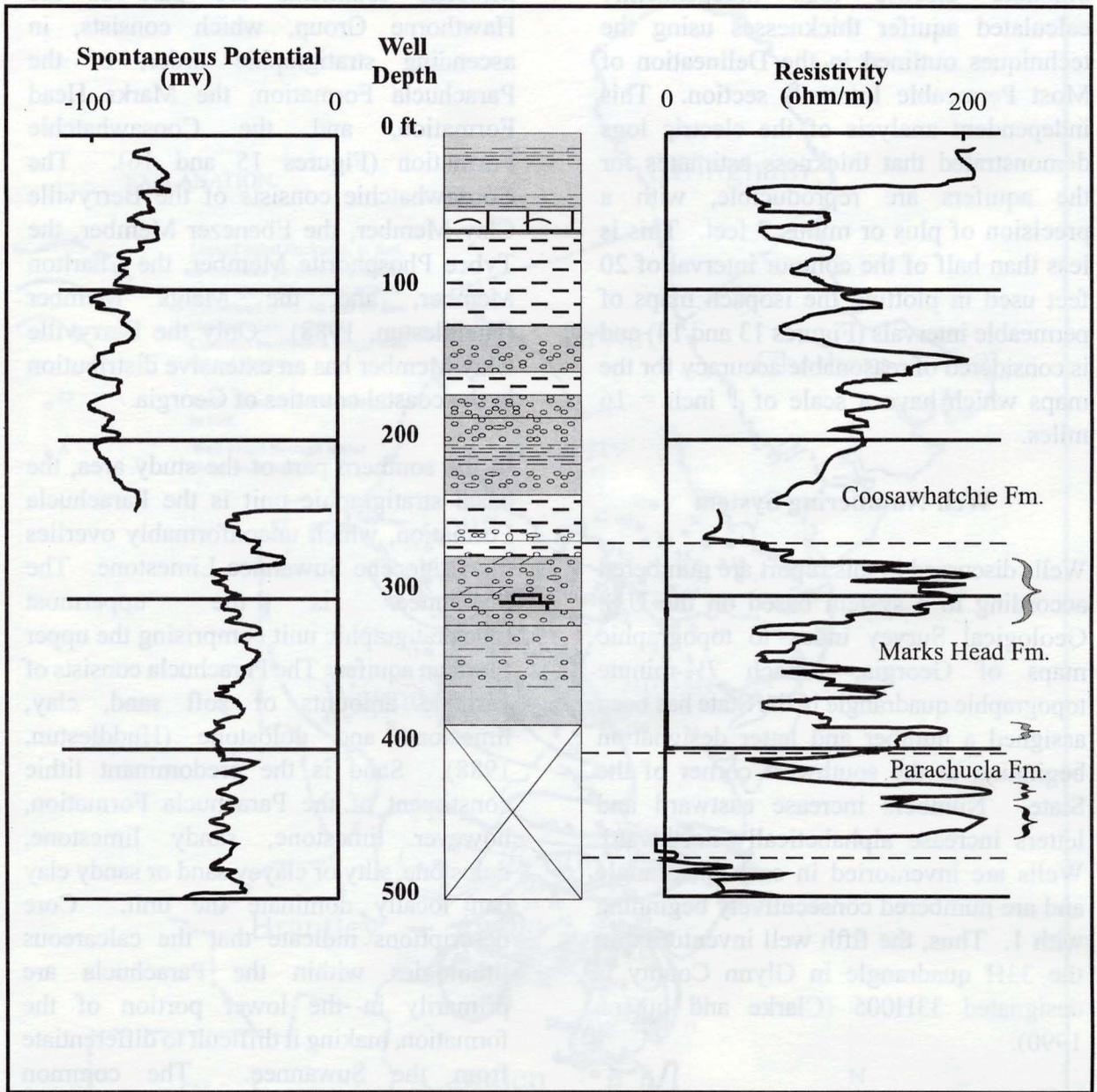
Figure 12: Stratigraphic column and electric logs of well 32K017, Wayne County.
