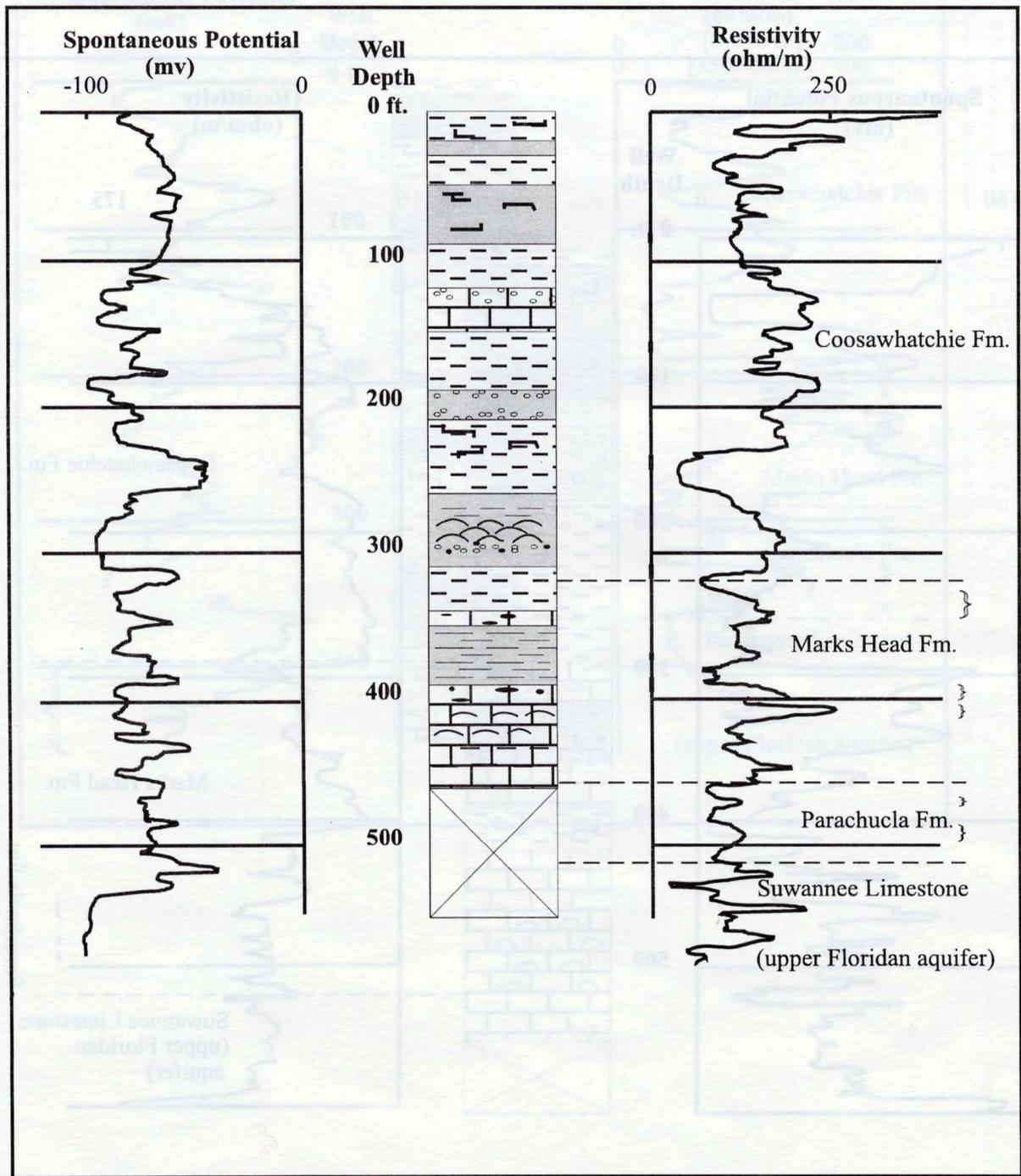
Figure 11: Stratigraphic column and electric logs of well 31L010, Wayne County.
