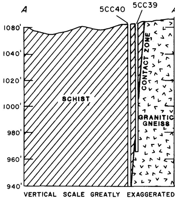
Figure 25. Well in contact zone between schist and granitic gneiss. Well 5CC39 yields 100 gallons per minute from the contact zone. Well 5CC40, which missed the contact zone, supplied about 1 gallon per minute.
