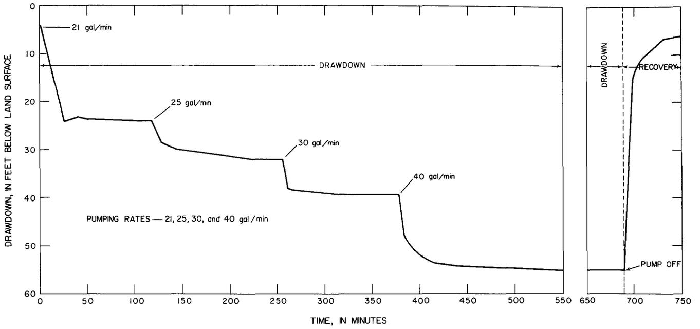
Figure 33. Drawdown and recovery curve for step drawdown test on test well 3 (9DD1).
