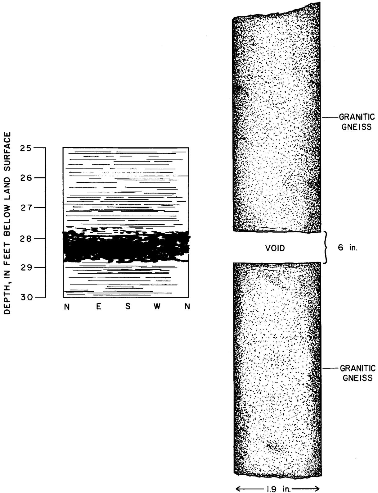
Figure 7. Comparison of televiwer image of horizontal water-bearing fracture with diagram of drill core, well 13DD90, Rockdale County.
