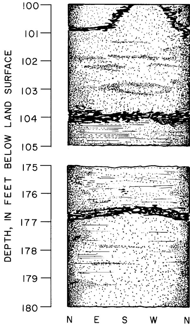
Figure 6. Televiewer image of non-water-bearing high-angle fracture at 100 feet, water-bearing horizontal fracture at 104 feet, and nearly horizontal water-bearing fracture at 176.5 feet, test well 2 (8CC8). Letters at bottom of image refer to compass quadrants.
