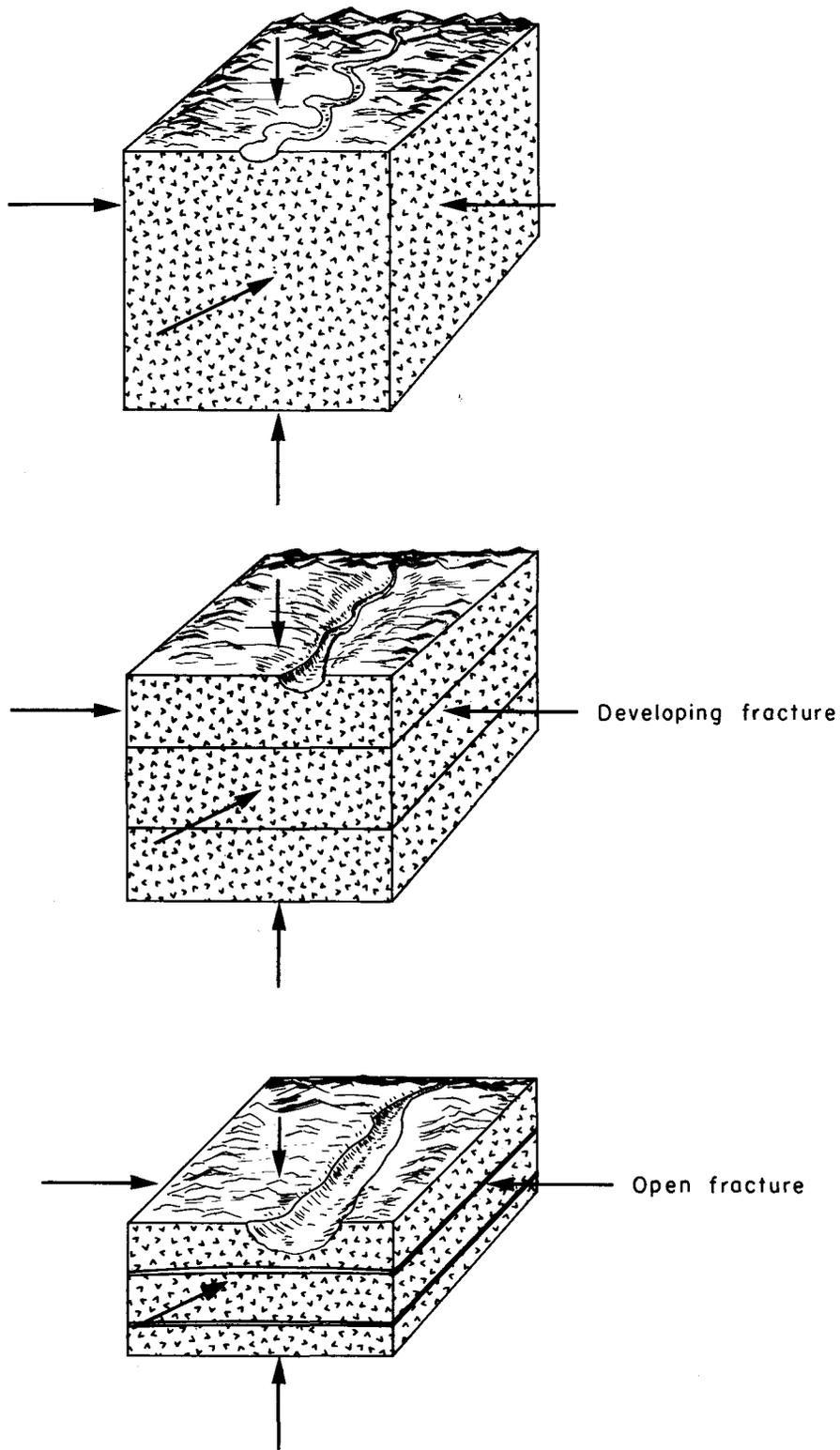
Figure 9. Stress relief fractures are believed to be caused by the upward expansion of the rock column in response to erosional unloading. Arrows represent the direction and their length represents strength of compressional stress.
