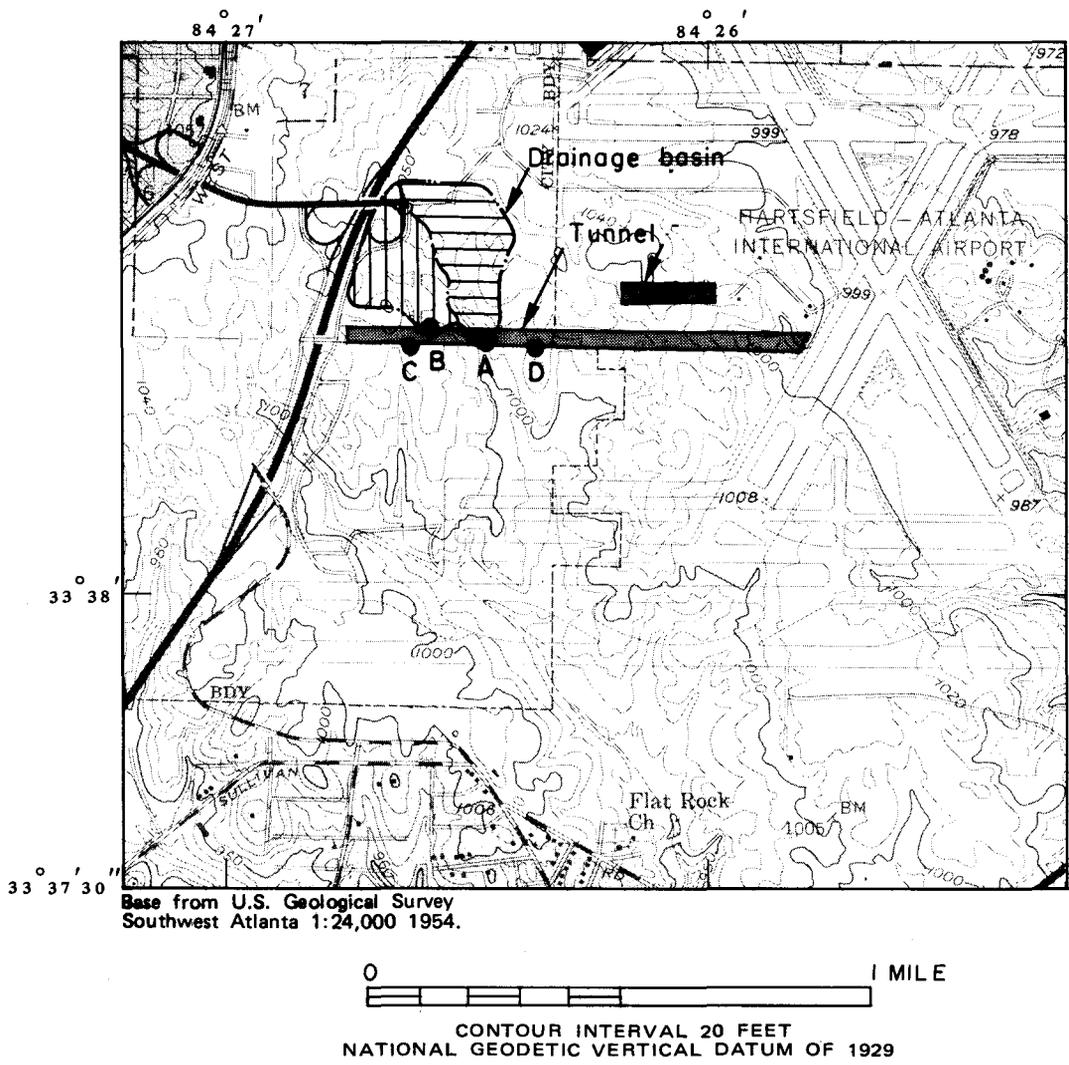
Figure 2. Well sites in the "people mover" tunnel area, Hartsfield-Atlanta International Airport. Sites A and B are downgradient from catchment areas supplying recharge; sites C and D are in interstream areas receiving little recharge.
